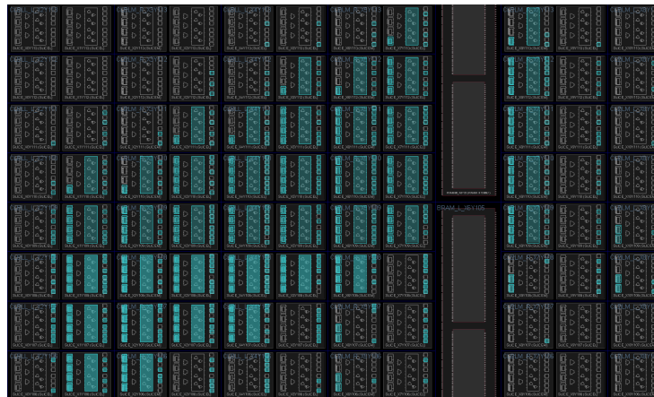
Figure 17. Implementation of the proposed 16 \times 16 pipelined multiplier (with an eight-stage pipeline using SRLs) showing the usage of LUT6s, CARRY4s and flip-flops.
