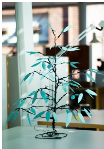
Figure 7. Talking Tree—a tree-shaped public display with interactive leaves made from sensitive colour paper.
