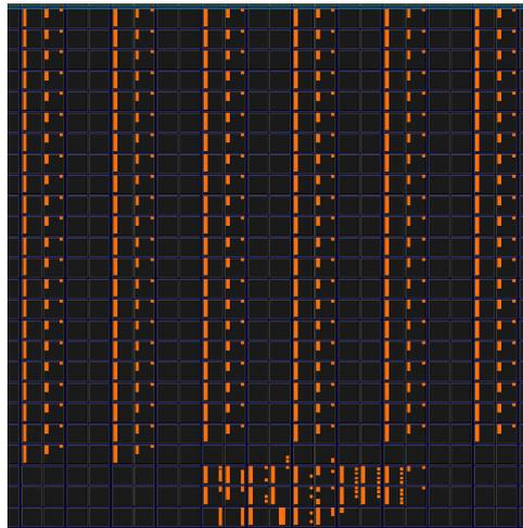
Figure 6. RO PUF manual placement overview.
