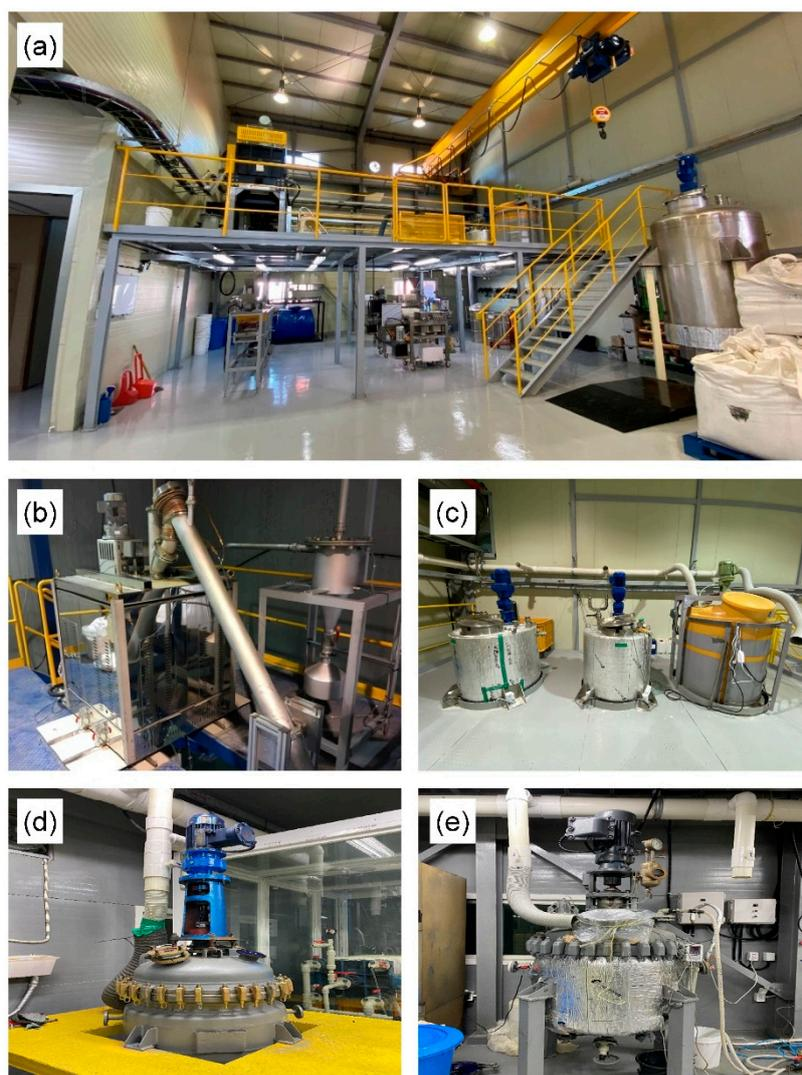
**Figure 11.** Photographs of (a) pilot-scale plant, (b) the furnace used for the continuous soda-melting reactions (100 L), (c) reactors for water leaching, desilication and precipitation (1 m<sup>3</sup>), (d) glass-lined reactor for a preparation of tungstic acid (100 L) and (e) glass-lined reactor for Ti leaching and hydrolysis (300 L).
