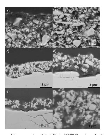
**Figure 4.** SEM images of the cross-sections of Ag-infiltrated LSCF films after reduction at 300 °C for 2 h in 5%  $H_2/Ar$ . Images were taken at the edge (left side, **a,c,e**) and center (right side, **b,d,f**) of each film. (**a**) and (**b**) Ag/LSCF<sub>com</sub>–SP (**c**) and (**d**) Ag/LSCF<sub>com</sub>–SC, and e) and f) Ag/LSCF<sub>syn</sub>–SC. Ag particles can be identified as brighter spots on the images.
