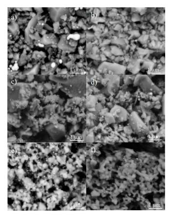
**Figure 3.** SEM images of the surface of Ag-infiltrated LSCF films after reduction at 300  $^{\circ}$ C for 2 h in 5% H<sub>2</sub>/Ar. Images were taken at the center (left side, **a**,**c**,**e**) and edge (right side, **b**,**d**,**f**) of each film. (**a**) and (**b**) Ag/LSCF<sub>com</sub>–SP (**c**) and (**d**) Ag/LSCF<sub>com</sub>–SC, and (**e**) and (**f**) Ag/LSCF<sub>syn</sub>–SC. Ag particles can be identified as brighter spots on the images.
