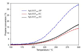
**Figure 8.** Catalytic performances of Ag-infiltrated LSCF layers. Test conditions:  $0.1\% C_3H_6/3.6\% O_2$  (He carrier, total flow 3 L h<sup>-1</sup>). The silver particles were reduced in situ at 300 °C for 2h in 5% H<sub>2</sub>/Ar (3 L h<sup>-1</sup>) prior to the test.
