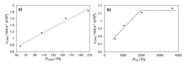
**Figure 10.** Catalytic rate on Ag/LSCF<sub>com</sub>–SP versus (a) partial pressure of propene (PO<sub>2</sub> = 3600 Pa) and (b) partial pressure of oxygen (PC<sub>3</sub>H<sub>6</sub> = 100 Pa). T = 300 °C.
