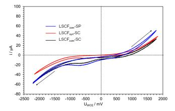
**Figure 7.** Comparison of the 20th cyclic voltammogram recorded at 300  $^{\circ}$ C in the reactive mixture on bare LSCF layers. The voltammograms are recorded between -2 V and +2 V with a scan rate of 10 mV/s.
