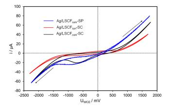
**Figure 9.** Comparison of the 20th cyclic voltammogram recorded at 300  $^{\circ}$ C in the reactive mixture on Ag-infiltrated LSCF layers. The voltammograms are recorded between -2 V and +2 V with a scan rate of 10 mV/s.
