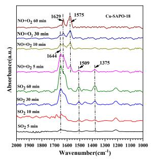
**Figure 9.** DRIFT spectra of the Cu-SAPO-18 sample exposed to 100 ppm SO<sub>2</sub>, followed by introduction of 500 ppm NO in the presence of O<sub>2</sub> at 150 °C.
