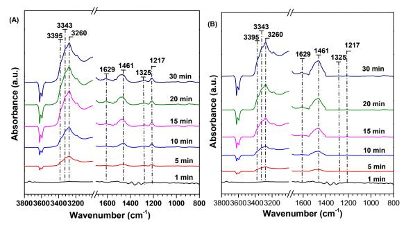
**Figure 5.** DRIFT spectra of NH<sub>3</sub> adsorption on (**A**) Cu-SAPO-18 and (**B**) Cu-SAPO-18-S at 150 °C for various time.
