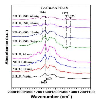
**Figure 8.** DRIFT spectra of the Ce-Cu-SAPO-18 sample exposed to 500 ppm NO in the presence of  $O_2$ , followed by introduction of 100 ppm SO<sub>2</sub> at 150 °C.
