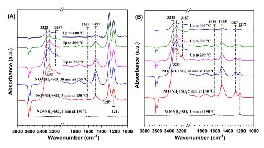
**Figure 11.** DRIFT spectra of (**A**) Cu-SAPO-18 and (**B**) Ce-Cu-SAPO-18 first exposed to 500 ppm NO + 500 ppm NH<sub>3</sub> + 100 ppm SO<sub>2</sub> in the presence of O<sub>2</sub> at 150 °C for various time, and then switched from the NO/NH<sub>3</sub>/SO<sub>2</sub>/N<sub>2</sub> mixture to only N<sub>2</sub> with the temperature being increased from 150 to 400 °C.
