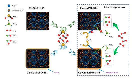
Scheme 1. Formation pathways of the bulk-like sulfates on the Ce-Cu-SAPO-18 sample.
