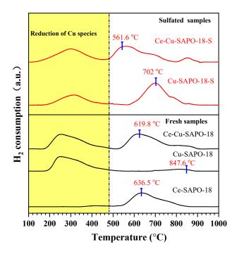
Figure 4. H<sub>2</sub>-TPR profiles of the fresh and sulfated samples.
