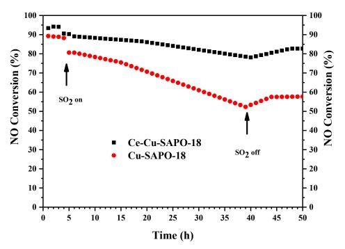
**Figure 2.** NO conversion as a function of reaction time over the Cu-SAPO-18 and Ce-Cu-SAPO-18 samples in the presence and absence of SO<sub>2</sub> at 300 °C. The reactant feed composition: 500 ppm NO, 500 ppm NH<sub>3</sub>, 100 ppm SO<sub>2</sub> (when used), 14 vol.%  $O_2$ , 5 vol.% H<sub>2</sub>O, and N<sub>2</sub> (balance).
