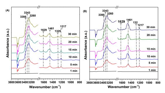
**Figure 6.** DRIFT spectra of NH<sub>3</sub> adsorption on (**A**) Ce-Cu-SAPO-18 and (**B**) Ce-Cu-SAPO-18-S at 150 °C for various times.
