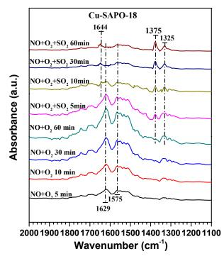
**Figure 7.** DRIFT spectra of the Cu-SAPO-18 sample exposed to 500 ppm NO in the presence of  $O_2$ , followed by introduction of 100 ppm SO<sub>2</sub> at 150 °C.
