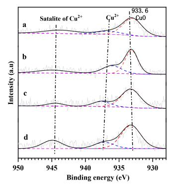
**Figure 3.** Cu 2p3/2 XPS spectra of the fresh and sulfated samples: (**a**) Cu-SAPO-18, (**b**) Cu-SAPO-18-S, (**c**) Ce-Cu-SAPO-18, and (**d**) Ce-Cu-SAPO-18-S.
