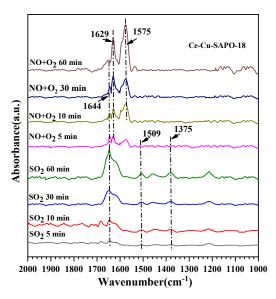
**Figure 10.** DRIFT spectra of the Ce-Cu-SAPO-18 sample exposed to 100 ppm SO<sub>2</sub>, followed by introduction of 500 ppm NO in the presence of  $O_2$  at 150 °C.
