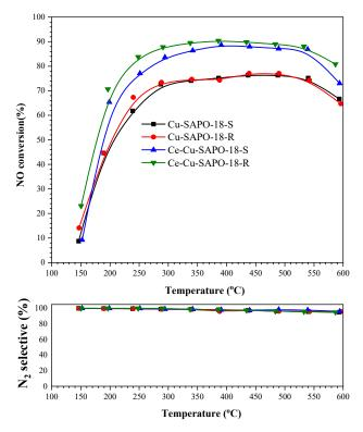
**Figure 12.** NO conversion and N<sub>2</sub> selectivity as a function of temperature for the NH<sub>3</sub>-SCR reaction over the Cu-SAPO-18-S, Cu-SAPO-18-R, Ce-Cu-SAPO-18-S and Ce-Cu-SAPO-18-R samples at a GHSV of 130,000  $h^{-1}$ . The reactant feed composition: 500 ppm NO, 500 ppm NH<sub>3</sub>, 14 vol.% O<sub>2</sub>, 5 vol.% H<sub>2</sub>O, and N<sub>2</sub> (balance).
