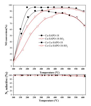
**Figure 1.** NO conversion and N<sub>2</sub> selectivity during the NH<sub>3</sub>-SCR reaction over the Cu-SAPO-18 and Ce-Cu-SAPO-18 samples at a GHSV of 130,000 h<sup>-1</sup>. The reactant feed composition: 500 ppm NO, 500 ppm NH<sub>3</sub>, 100 ppm SO<sub>2</sub> (when used), 14 vol.% O<sub>2</sub>, 5 vol.% H<sub>2</sub>O, and N<sub>2</sub> (balance).
