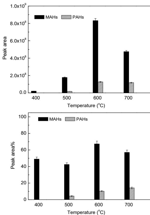
**Figure 5.** Effects of reaction temperature on the yield and selectivity of aromatics. (10Mo/ZSM-5, catalyst/biomass mass ratio = 10).
