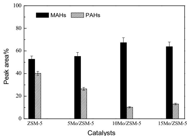
**Figure 4.** Distribution of aromatics produced from catalytic fast pyrolysis (CFP) of biomass over different catalysts (T = 600 °C, catalyst/biomass mass ratio = 10).
