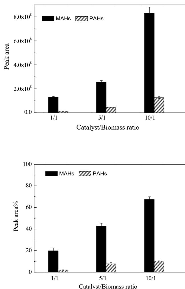
**Figure 6.** Effects of catalyst/biomass mass ratios on the yields and selectivity of aromatics. (10Mo/ZSM-5, T = 600 °C).
