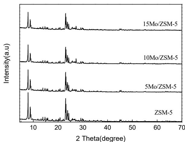
**Figure 1.** X-ray diffraction (XRD) patterns of the ZSM-5 and Mo/ZSM-5 catalysts.
