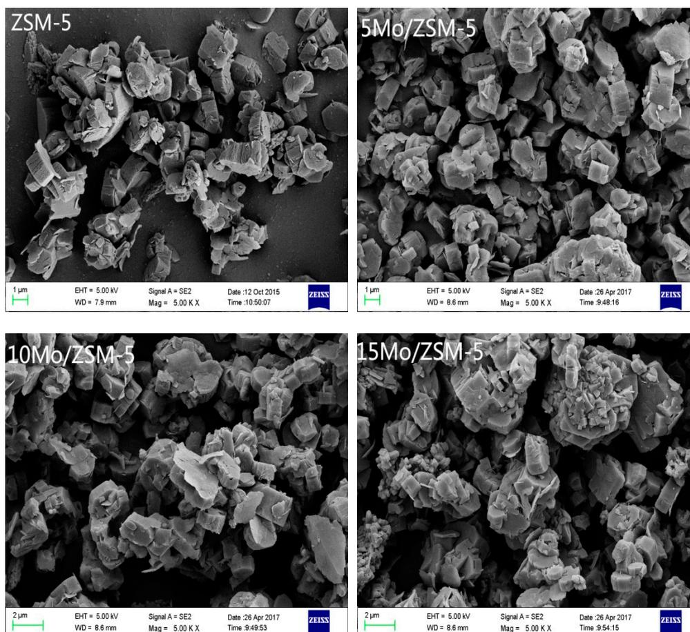
**Figure 2.** The scanning electron microscopy (SEM) images of the ZSM-5 and Mo/ZSM-5 catalysts.
