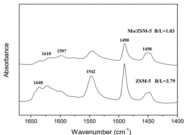
**Figure 3.** Pyridine infrared spectroscopy (Py-IR) of the ZSM-5 and Mo/ZSM-5 catalysts.
