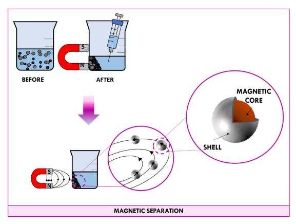
**Figure 5.** Schematic representation of the magnetic separation.
