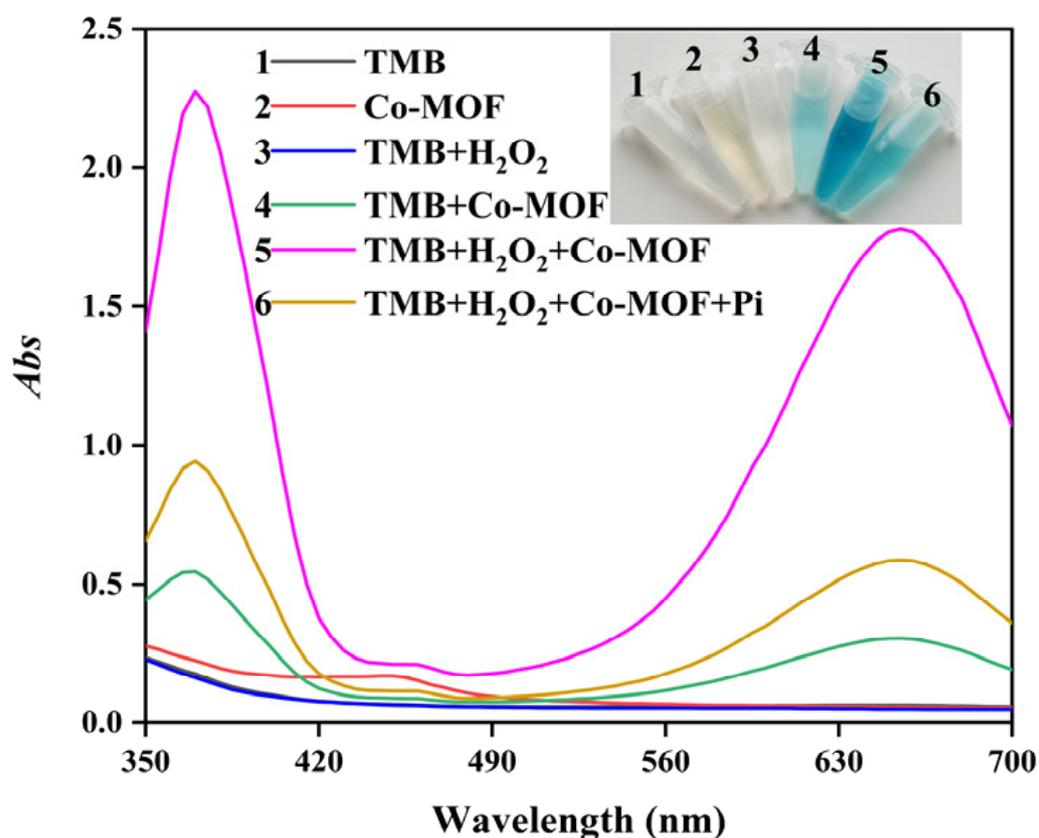
**Figure 5.** The absorption spectra and corresponding color change of diverse catalytic reaction systems.
