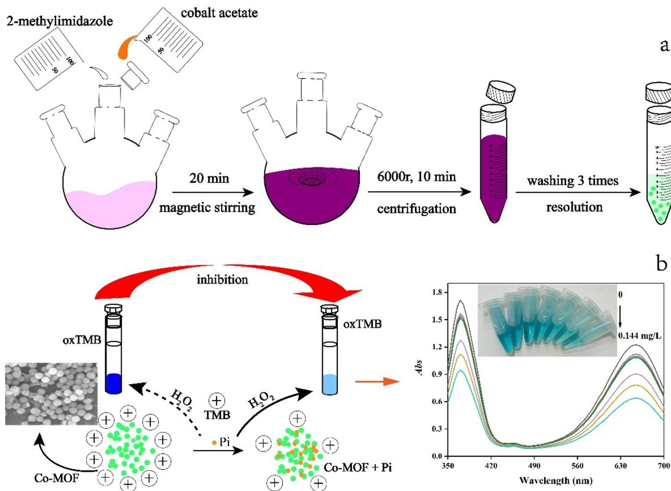
**Scheme 1.** Diagram for synthesis process of Co-MOF (a), and colorimetric sensing of Pi based on the target-induced differential peroxidase-like activity changes of Co-MOF (b).
