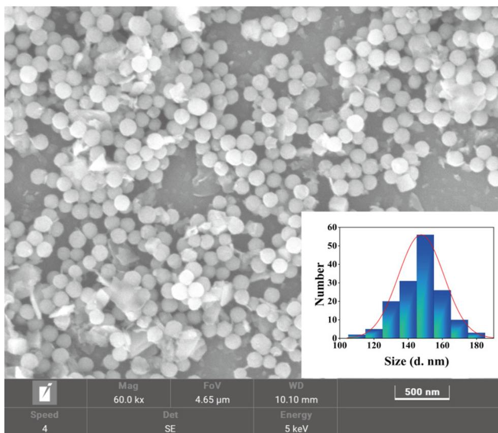
**Figure 1.** The SEM image and the size distribution (inserted).
