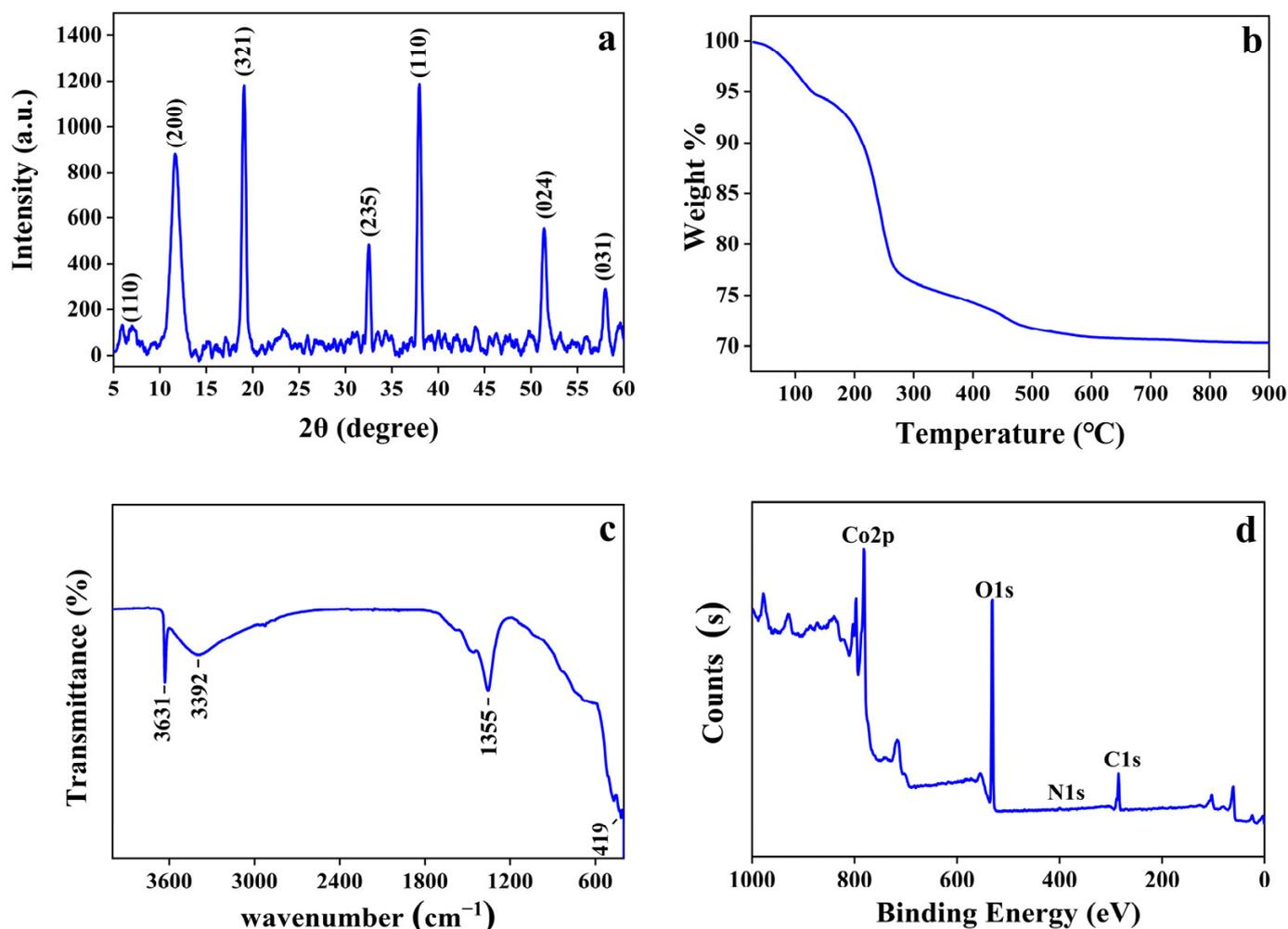
**Figure 2.** The XRD pattern (a), TG curve (b), FTIR spectrum (c), and XPS diagram (d) of Co-MOF.
