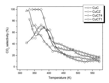
**Figure 4.** CO<sub>2</sub> production during the CO-TPR runs performed with a tubular reactor over the indicated samples. A CuO reference sample prepared by microemulsion has been included for comparative purpose. Note: This figure is reproduced with permission from [48]. Copyright © 2009, Elsevier Inc.
