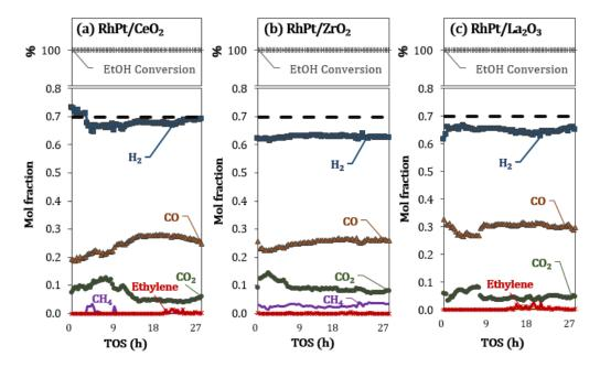
**Figure 2.** Product distribution (H<sub>2</sub>, CO, CO<sub>2</sub>, CH<sub>4</sub>, and ethylene) as a function of time on stream (TOS) on reduced (**a**) RhPt/CeO<sub>2</sub>; (**b**) RhPt/ZrO<sub>2</sub>; and (**c**) RhPt/La<sub>2</sub>O<sub>3</sub>. Dashed line: H<sub>2</sub> equilibrium. Reaction conditions: S/E = 3 and GHSV = 70,600 h<sup>-1</sup> at 700 °C.
