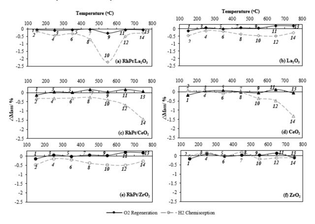
**Figure 3.** Oxidation in  $1\%O_2/N_2$  (No. 1, 3, 5, 7, 9, 11, 13) and reduction in  $4\%H_2/N_2$  (No. 2, 4, 6, 8, 10, 12, 14) as a function of temperature in a thermogravimetric analysis of fresh RhPt supported catalysts (**a**, **c**, **e**) and catalyst supports (**b**, **d**, **f**).
