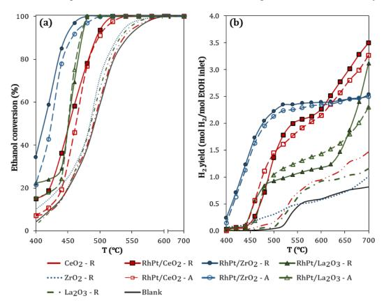
**Figure 1.** (a) Ethanol conversion (XEtOH) and (b)  $H_2$  yield as a function of temperature for reduced (R) and aged (A) RhPt/CeO<sub>2</sub>, RhPt/ZrO<sub>2</sub>, and RhPt/La<sub>2</sub>O<sub>3</sub>. Reaction conditions: S/E = 3 and  $GHSV = 70600 \text{ h}^{-1}$ . Aged samples obtained after 27 h TOS at 700 °C.
