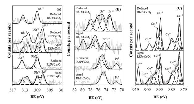
**Figure 6.** XPS spectra of (a) Rh  $3d_{5/2}$ ; (b) Pt  $7f_{7/2}$ ; and (c) Ce  $3d_{3/2}$  and  $3d_{5/2}$  for reduced and aged catalysts.
