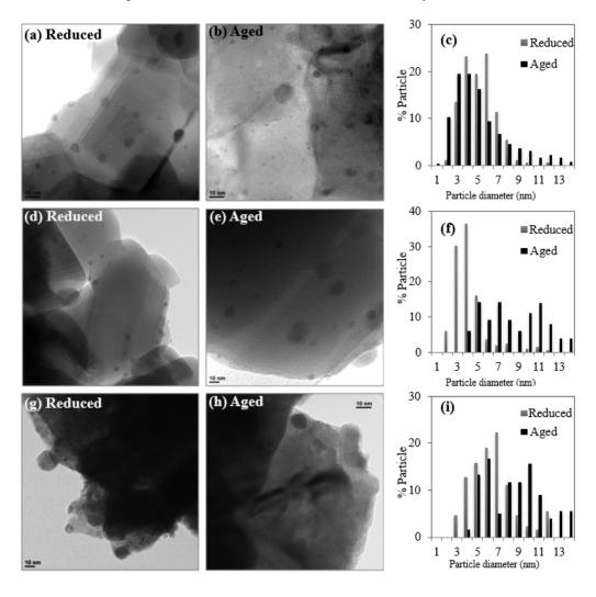
**Figure 4.** TEM images and particle size distribution histograms of reduced and aged catalysts: (a), (b), and (c) RhPt/CeO<sub>2</sub>; (d), (e), and (f) RhPt/ZrO<sub>2</sub>; (g), (h), and (i) RhPt/La<sub>2</sub>O<sub>3</sub>.
