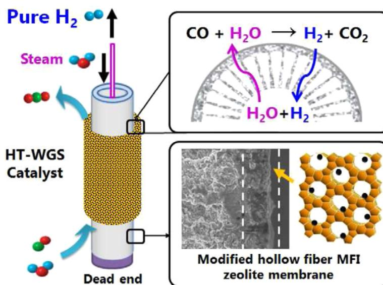
**Figure 6.** Schematic illustration of a WGS membrane reactor with modified hollow fibre MFI zeolite membrane swept by steam applied in a counter-diffusion towards the reaction side. Reprinted with permission from [157]. Copyright (2015) John Wiley and Sons.
