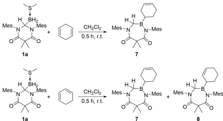
**Scheme 6.** Hydroboration of cyclic olefins with **1a**.
