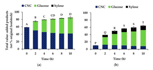
**Figure 2.** Total value-added products (CNC and sugars, wt % original feedstock) extracted from (a) filter paper and (b) wood pulp, via enzyme-mediated CNC production process. Error bars represent standard deviation of the total value-added products (wt % original feedstock). Bars that are denoted by non-identical letters are significantly different (p < 0.05). Means and standard deviations for CNC yield from filter paper, cellulase cocktail treated for 10 h, were calculated from duplicates.
