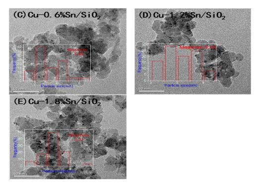
**Figure 4.** The TEM images of the reduced catalysts: (**A**) Cu/SiO<sub>2</sub>, (**B**) Cu-0.3%Sn/SiO<sub>2</sub>, (**C**) Cu-0.6%Sn/SiO<sub>2</sub>, (**D**) Cu-1.2%Sn/SiO<sub>2</sub> and (**E**) Cu-1.8%Sn/SiO<sub>2</sub>.
