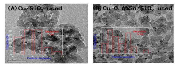
Figure 10. TEM images of used catalysts: (A) Cu/SiO<sub>2</sub>-used (130 h) and (B) Cu-0.6%Sn/SiO<sub>2</sub>-used (200 h).
