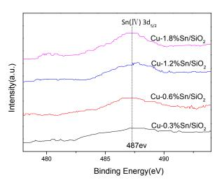
**Figure 7.** X-ray photoelectron spectroscopy (XPS) spectra of Sn  $3d_{5/2}$  of Cu/SiO<sub>2</sub> and Cu-xSn/SiO<sub>2</sub> catalysts under an 8 h reaction.
