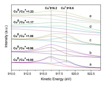
**Figure 9.** Curve fitting results of the Cu LMM XAES spectra of catalysts: (a) Cu/SiO<sub>2</sub>, (b) Cu-0.3%Sn/SiO<sub>2</sub>, (c) Cu-0.6%Sn/SiO<sub>2</sub>, (d) Cu-1.2%Sn/SiO<sub>2</sub> and (e) Cu-1.8%Sn/SiO<sub>2</sub> after 8 h reaction.
