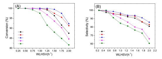
**Figure 5.** Comparison of dimethyl oxalate (DMO) conversion (**A**) and ethylene glycol (EG) selectivity (**B**) in Cu/SiO<sub>2</sub> and Cu-*x*Sn/SiO<sub>2</sub> catalysts with varied WLHSVs.
