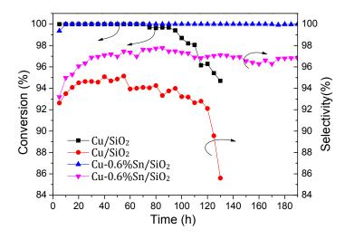
**Figure 6.** Long experimental periods of Cu/SiO<sub>2</sub> and Cu-x0.6%Sn/SiO<sub>2</sub> catalysts. The reaction conditions were 2.5 MPa  $H_2$ , 200 °C,  $H_2$ /DMO ratio of 90 and WLHSV of 1  $h^{-1}$ .
