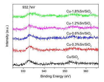
Figure 8. XPS spectra of Cu 2p of Cu/SiO<sub>2</sub> and Cu-xSn/SiO<sub>2</sub> catalysts under an 8 h reaction.
