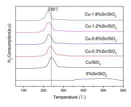
**Figure 2.** H<sub>2</sub>-temperature-programmed reduction of 5% Sn/SiO<sub>2</sub>, Cu/SiO<sub>2</sub> and Cu–xSn/SiO<sub>2</sub> catalysts after calcination at 300 °C.
