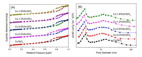
**Figure 1.** N<sub>2</sub> adsorption–desorption profiles (**A**) and Barrett–Joyner–Halenda (BJH) pore-size distribution curves (**B**) of calcined Cu/SiO<sub>2</sub> and Cu-*x*Sn/SiO<sub>2</sub> catalysts.
