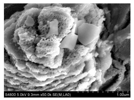
Figure S3. FE-SEM image of top view of the PCT film.
