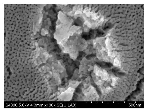
Figure S7. FE-SEM image of small cracks in the Figure 1A.
