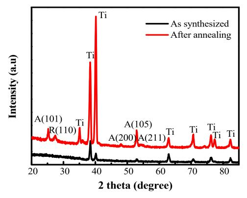
**Figure S9.** XRD patterns of the PCT films. Specific diffraction peaks for anatase (JCPDS#21–1272) and rutile (JCPDS#21–1276) are labeled according to A(hkl) and R(hkl), respectively.
