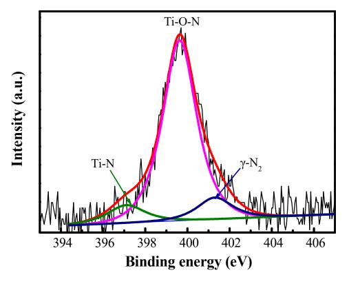
Figure S12. N 1s XPS spectrum of the PCT film.
