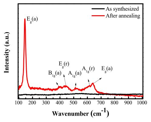
**Figure S10.** Raman scattering patterns of the PCT films, where the anatase and rutile vibration modes are labeled according to mode (a) and mode (r), respectively.
