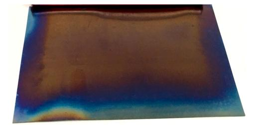
**Figure S17.** Pictures for the large-scale PCT films prepared by different anodization conditions. A laptop was used as a reference.
