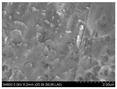
**Figure S2.** FE-SEM images of the TiO<sub>2</sub> film anodized in the electrolyte of magnesium nitrate solution (100 mg L<sup>-1</sup>, 50 mL) at 60 V for 2 min.
