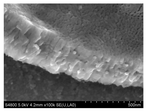
Figure S8. FE-SEM image of TiO<sub>2</sub> fragment washed up by O<sub>2</sub> gas.
