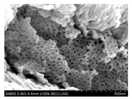
Figure S5. FE-SEM image of cracks on the oxide layer.
