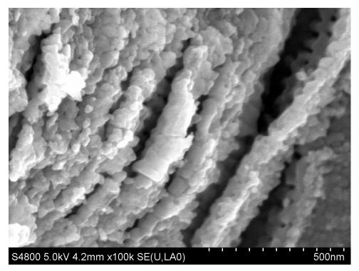
Figure S4. FE-SEM image of layer structure of the PCT film.
