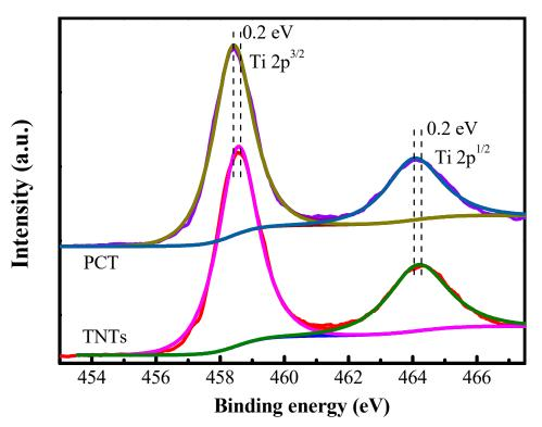
Figure S13. Ti 2p XPS spectra of the PCT film and TNTs.
