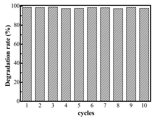
**Figure S16.** Stability test of methyl orange degradation for ten cycles under natural sunlight ( $C_{MO}$  = 20 mg L<sup>-1</sup>,  $V_{MO}$  = 40 mL).
