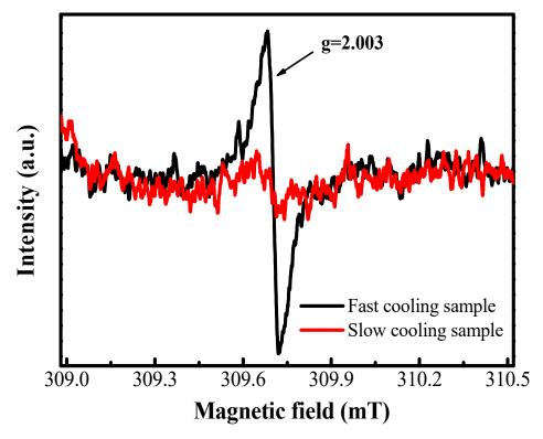
Figure S15. ESR spectra of PCT film with different cooling styles after calcination at 723 K for 2 h.
