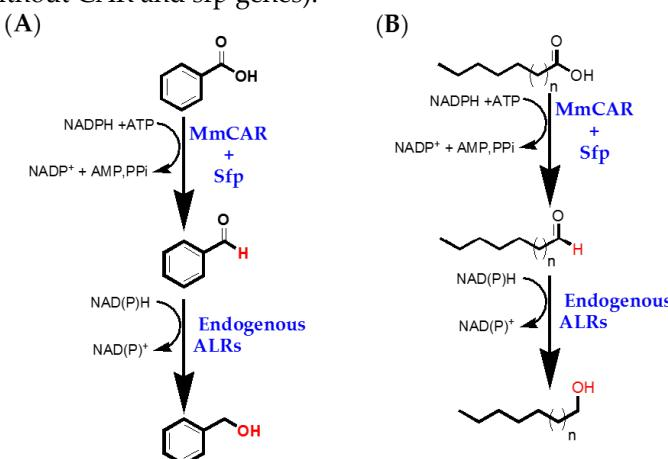
**Figure S4.** Proposed reaction scheme for the biosynthesis of benzyl alcohol and fatty alcohols (C<sub>8</sub>-C<sub>16</sub>).
