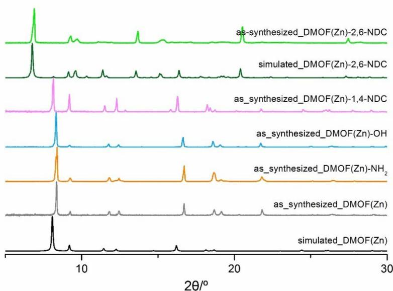
**Figure 3.** Powder X-ray diffraction (PXRD) patterns of DMOFs with different functionalities on the benzene-1,4-dicarboxylic acid (BDC) ligand.
