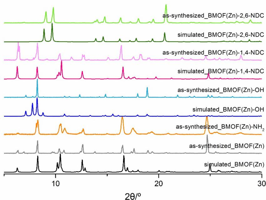
**Figure 4.** PXRD patterns of BMOFs (BPY MOFs) with different functionalities on the BDC ligand.
