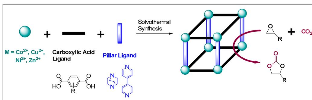
**Figure 1.** Three components in pillared metal-organic frameworks (MOFs) and CO<sub>2</sub> cycloaddition.
