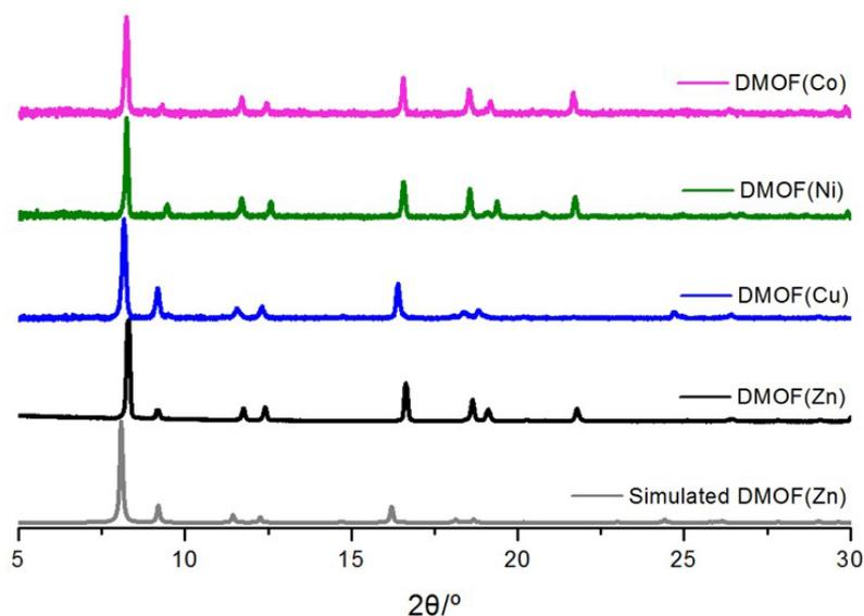
**Figure 2.** Powder X-ray diffraction (PXRD) patterns of DMOFs with different metal sources.
