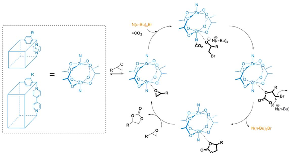
**Scheme 2.** Proposed reaction mechanism for CO<sub>2</sub> cycloaddition-catalyzed by pillared MOFs.
