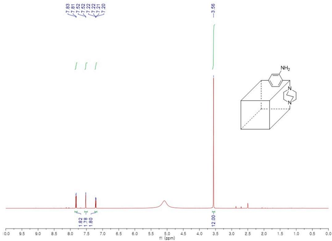
Figure S2.  $^1\text{H}$  NMR of DMOF(Zn)- $\text{NH}_2$  after acid digestion.
