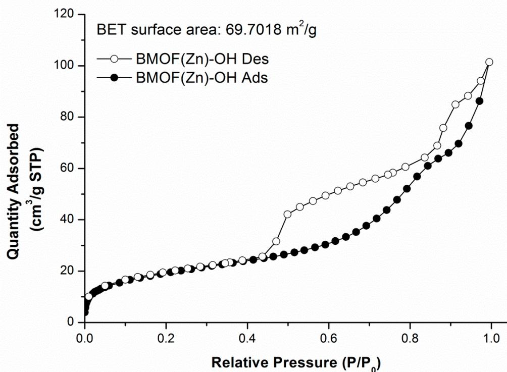
Figure S14. N<sub>2</sub> full isotherm (77 K) for BMOF(Zn)-OH.
