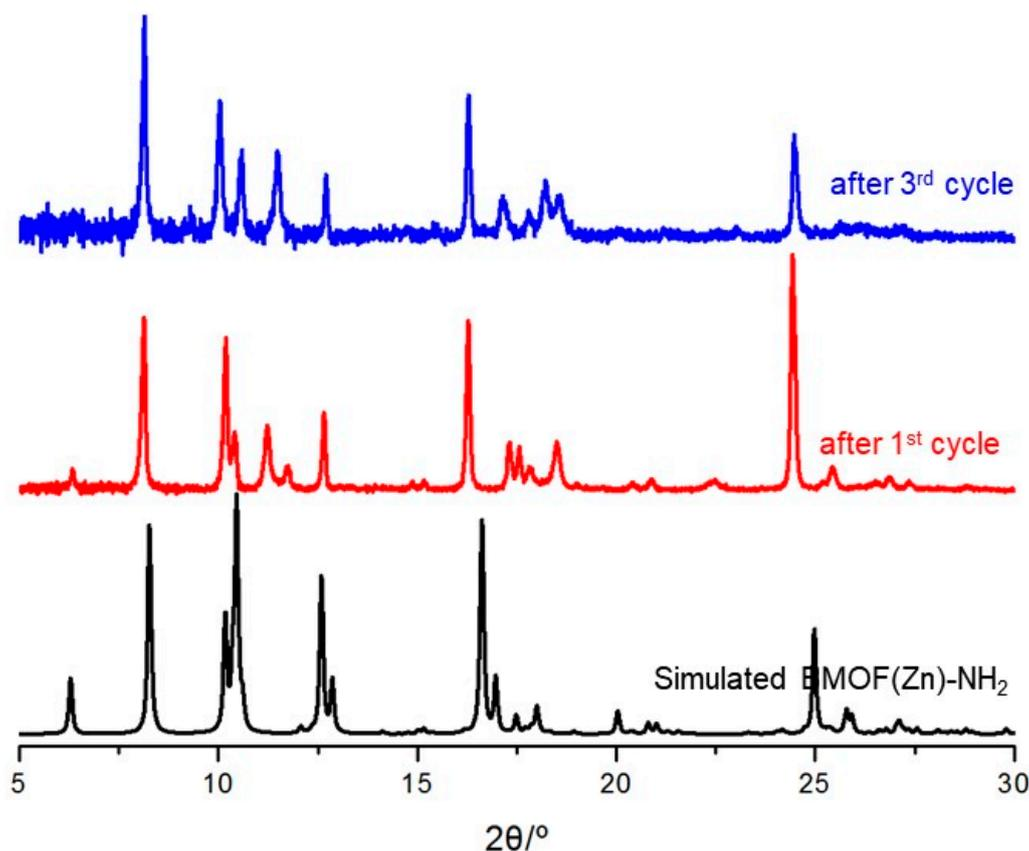
**Figure S16.** PXRD patterns of BMOF(Zn)-NH<sub>2</sub> before and after reaction.
