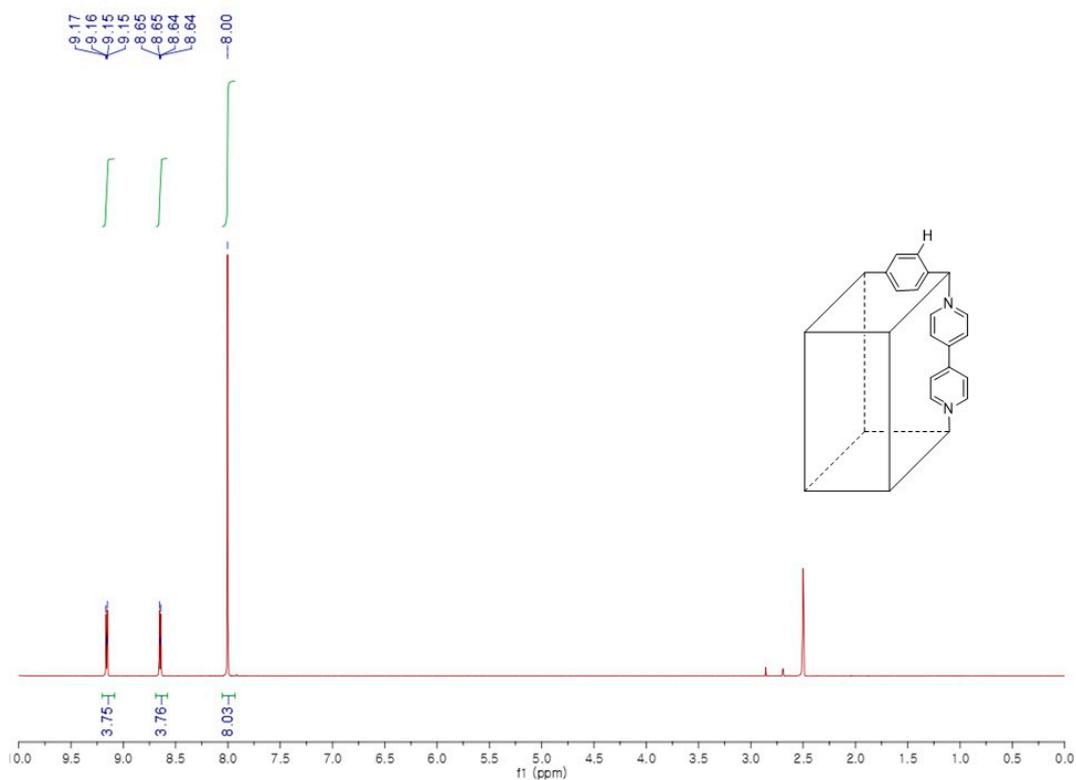
Figure S7.  $^1\text{H}$  NMR of BMOF(Zn) after acid digestion.
