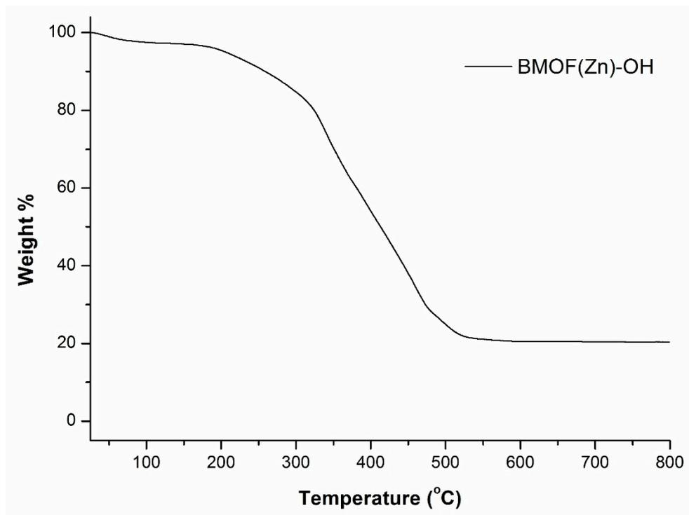
Figure S15. Thermogravimetric analysis of BMOF(Zn)-OH.
