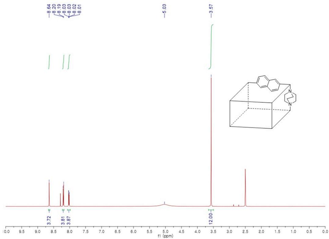
**Figure S5.**  $^1\text{H}$  NMR of DMOF(Zn)-1,5-NDC after acid digestion.
