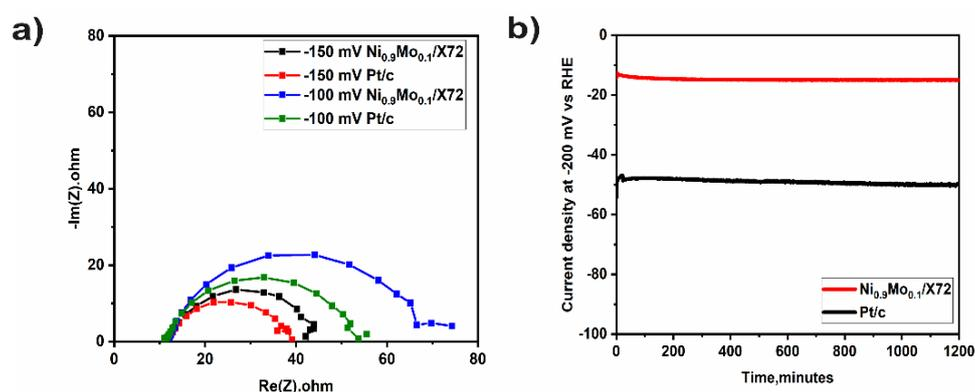
**Figure 5.** (a) Nyquist plot of Ni<sub>0.9</sub>Mo<sub>0.1</sub> and Pt/C in 1 M KOH at −150 and 150 mV vs. RHE (b) Chronoamperometry of Ni<sub>0.9</sub>Mo<sub>0.1</sub> and Pt/C for 24 h in 1 M KOH.
