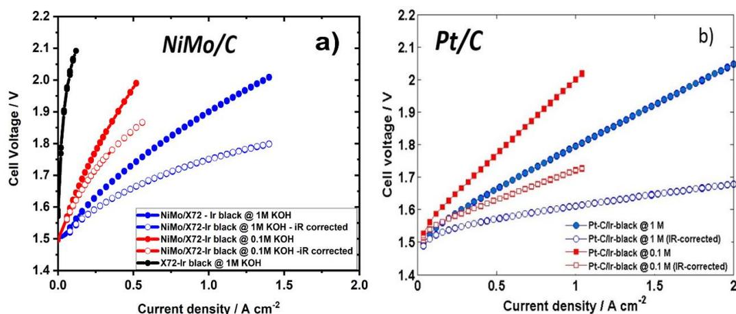
**Figure 7.** Polarization curves in both  $1 \text{ M}$  and  $0.1 \text{ M KOH}$  at  $50 \text{ }^\circ\text{C}$ . (a) A  $5 \text{ mg cm}^{-2}$  NiMo loading compared to (b) a  $1 \text{ mg cm}^{-2}$  Pt. Cell active area:  $25 \text{ cm}^{-2}$ . Both CCMs using  $3 \text{ mg cm}^{-2}$  Ir-black.
