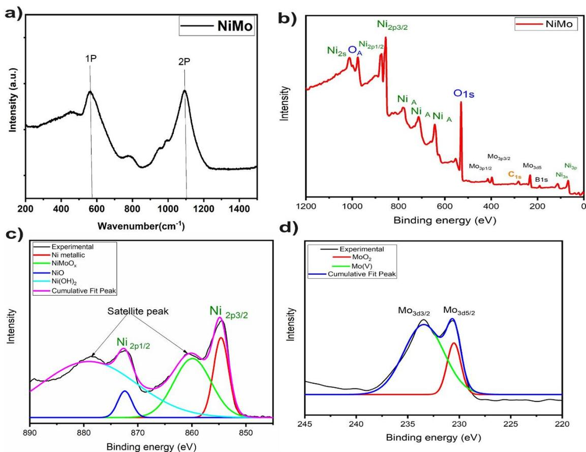
**Figure 3.** (a) Raman spectrum of  $\text{Ni}_{0.9}\text{Mo}_{0.1}$  nanosheets, (b) X-ray photoelectron spectroscopy (XPS) spectrum of  $\text{Ni}_{0.9}\text{Mo}_{0.1}$  nanosheets, (c) XPS peak fitting of Nickel peaks (d) XPS peak fitting of Mo peaks.
