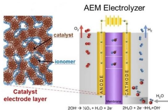
**Figure 1.** Catalyst electrode layer and membrane electrode assembly for anion exchange membrane (AEM) electrolyzer, where the catalyst is mixed with an ionomer, Reprinted from Artyushkova et al., License Number 4406040674790 [14].
