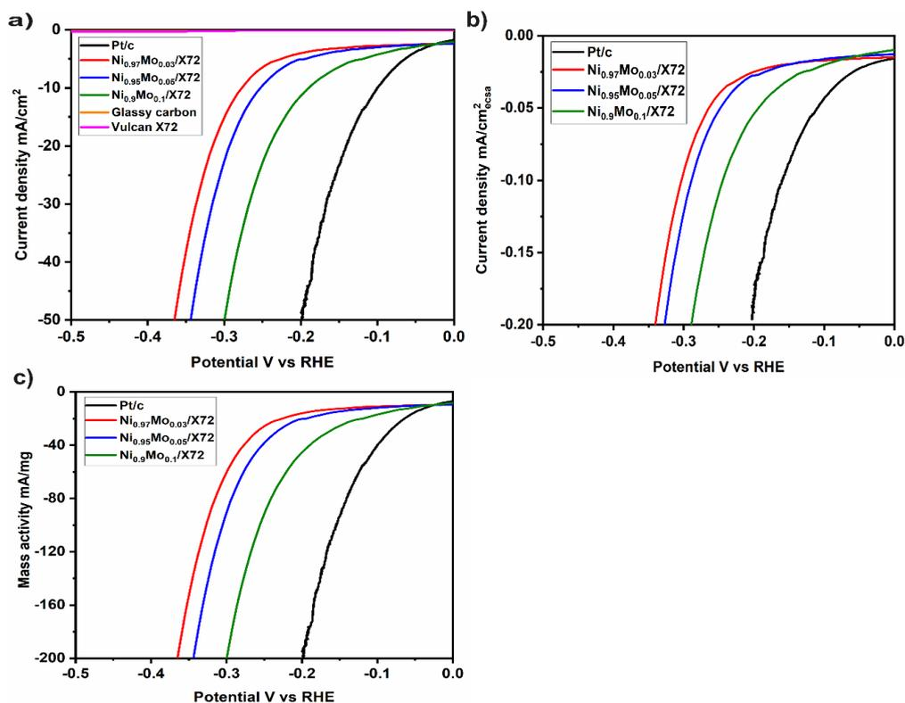
**Figure 4.** Linear sweep voltammetry (LSV) of NiMo with different Mo composition and Pt/C normalized to (a) geometric surface area and (b) electrochemical surface area and (c) mass loading.
