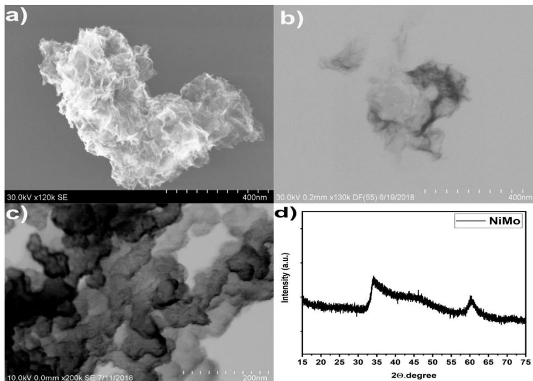
**Figure 2.** (a) SEM image of  $\text{Ni}_{0.9}\text{Mo}_{0.1}$  nanosheets, (b) Inverted dark field scanning transmission electron microscopy (STEM)  $\text{Ni}_{0.9}\text{Mo}_{0.1}$  nanosheets (c)  $\text{Ni}_{0.9}\text{Mo}_{0.1}$  supported in Vulcan XC72 prepared by chemical reduction, (d) X-ray diffraction pattern of  $\text{Ni}_{0.9}\text{Mo}_{0.1}$  nanosheets.
