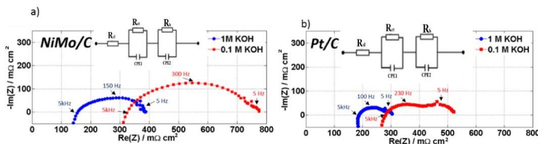
**Figure 6.** Electrochemical impedance is taken at 0.4 A in both 1 M and 0.1 M KOH at 50 °C. (a) A 5 mg cm<sup>-2</sup> NiMo loading compared to (b) a 1 mg cm<sup>-2</sup> Pt. Cell active area: 25 cm<sup>-2</sup>. Both catalyst coated membranes (CCMs) using 3 mg cm<sup>-2</sup> Ir-black. The impedance data represented by symbols and the fitted impedance data represented by a solid line.
