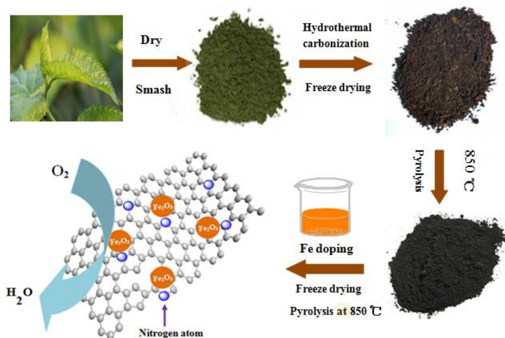
Scheme 1. The schematic illustration of the preparation process for \text{Fe}_2\text{O}_3/\text{N-PCs-850} nanoporous structures material.
