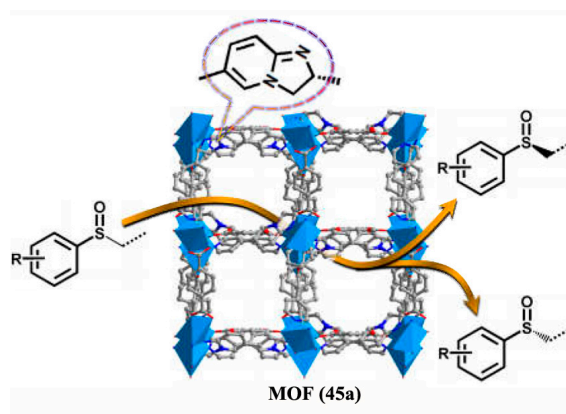
Figure 15. Enantioseparation of racemic sulfoxides by a Zn-DHIP MOF (45a). Reproduced from [110] with permission from the American Chemical Society.
