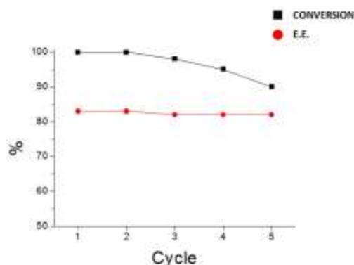
**Figure 2.** Enantiomeric excess (E.E.) variations and conversion values measured after 3 h by recycling **1-Mn** in the epoxidation of 1,2-dihydronaphthalene. Reaction conditions are reported in Entry 9 of Table 1.
