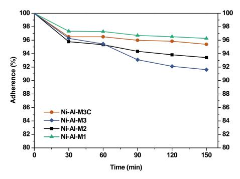
Figure 2. Adherence tests applied to the structured catalysts.
