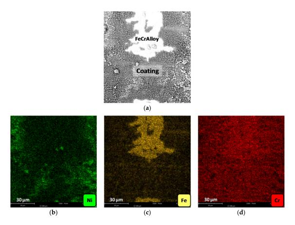
**Figure 5.** Mappings in an area of the Ni-Al-M1 structured catalyst: (a) SEM micrograph of the studied area, (b) Ni mapping, (c) Fe mapping and (d) Cr mapping.
