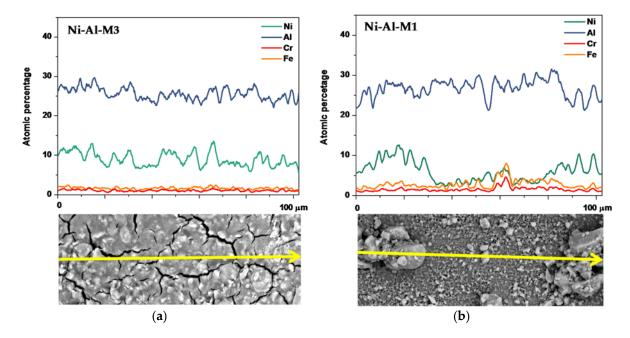
**Figure 4.** Linear mappings applied to (a) Ni-Al-M3 and (b) Ni-Al-M1 catalytic systems in the intermediate area of the valley.
