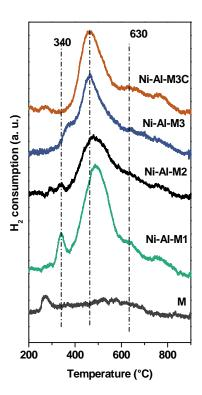
Figure 7. TPR profiles of the structured catalysts and a FeCrAlloy® sheet calcined at 900 °C for 22 h (M).
