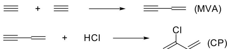
**Scheme 1.** C<sub>2</sub>H<sub>2</sub>-based process for 2-chloro-1,3-butadiene (CP) production.
