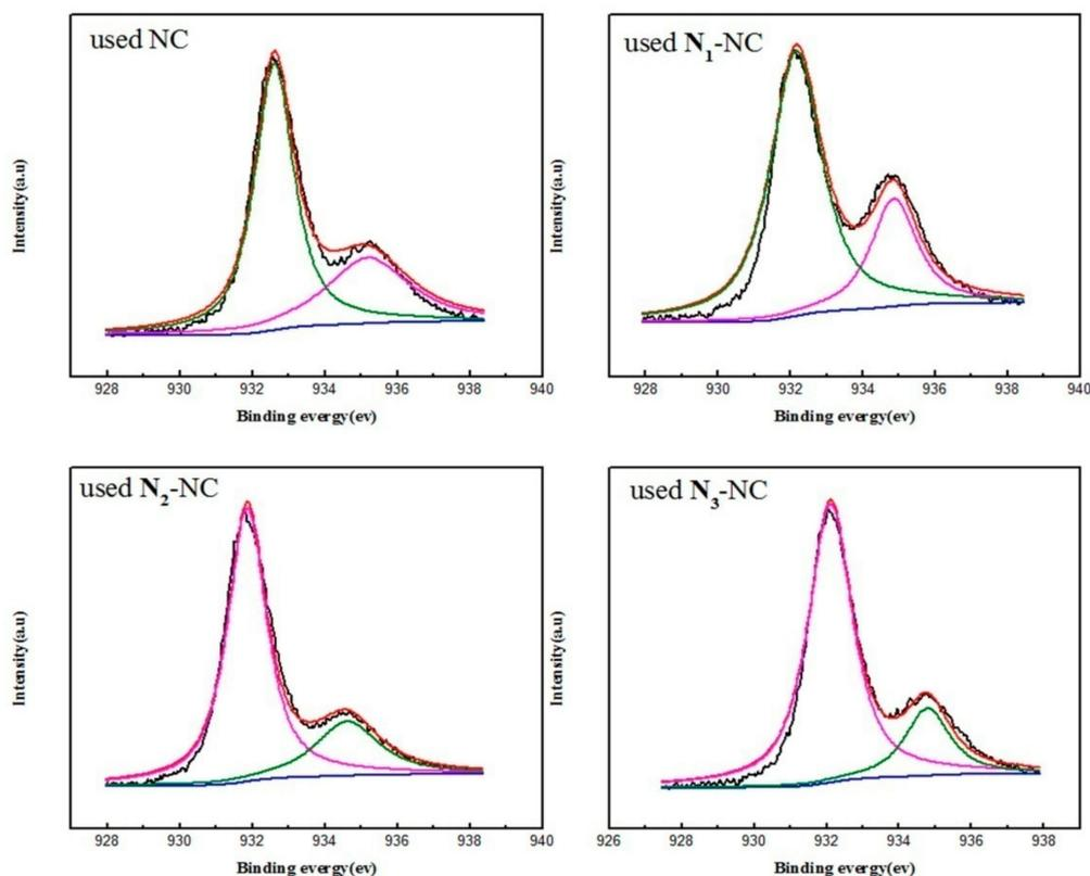
Figure 9. High-resolution XPS spectra of Cu  $2p_{3/2}$  of the fresh and used catalysts.
