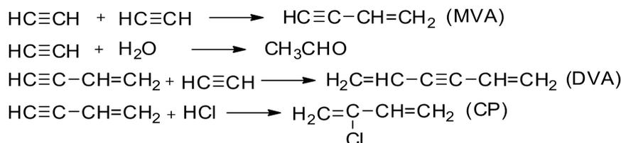
**Scheme 2.** The gas phase products of C<sub>2</sub>H<sub>2</sub> dimerization.
