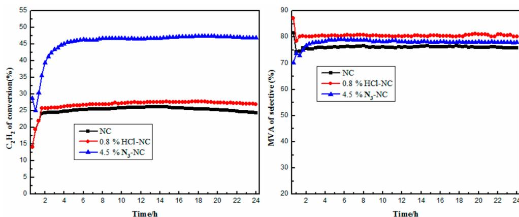
**Figure 2.** Lifetime testing of NC, 4.5% N<sub>3</sub>-NC and 0.8% HCl-NC.**Table 2.** Effect of NC, 4.5% N<sub>3</sub>-NC and 0.8% HCl-NC on acetylene conversion and MVA selectivity in acetylene dimerization.
