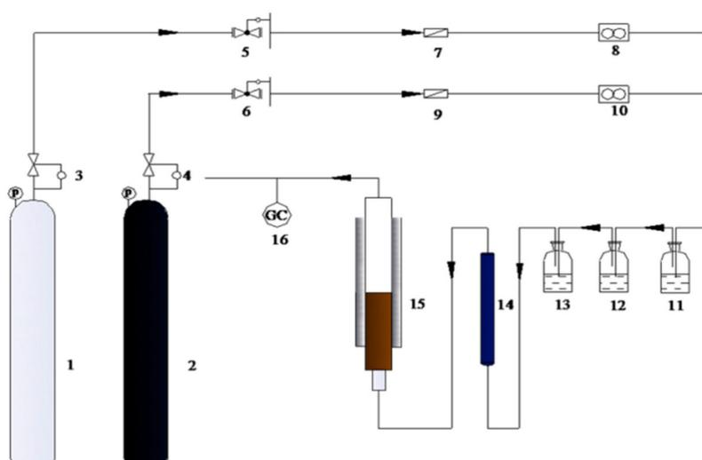
**Figure 11.** Schematic diagram of the C<sub>2</sub>H<sub>2</sub> dimerization system: 1 C<sub>2</sub>H<sub>2</sub>; 2 N<sub>2</sub>; 3,4 partial pressure valve; 5,6 check valve; 7,9 gas filter; 8,10 mass flow controller; 11 K<sub>2</sub>Cr<sub>2</sub>O<sub>7</sub> solution; 12 Na<sub>2</sub>S<sub>2</sub>O<sub>4</sub> solution; 13 NaOH solution; 14 drying tube; 15 reactor; 16 Gas Chromatograph (GC-2014C).
