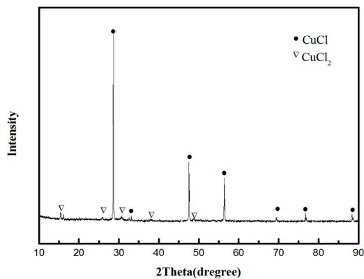
Figure 6. XRD study of heating product (450 °C) of the crystals.
