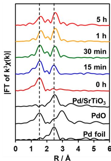
**Figure 5.** Fourier transforms of  $k^3$ -weighted Pd K-edge EXAFS spectra for PdCrO<sub>x</sub>/SrTiO<sub>3</sub> prepared for various time periods (0–5 h). Data for Pd foil, PdO and Pd/SrTiO<sub>3</sub> are shown as references.
