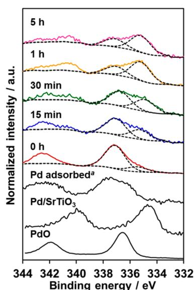
**Figure 6.** The XPS Pd 3d spectra for PdCrO<sub>x</sub>/SrTiO<sub>3</sub> prepared at various time periods (0–5 h). Data for PdO and Pd/SrTiO<sub>3</sub> are shown as references. <sup>a</sup> Pd precursor (Na<sub>2</sub>PdCl<sub>4</sub>·3H<sub>2</sub>O) adsorbed on SrTiO<sub>3</sub> under dark conditions.
