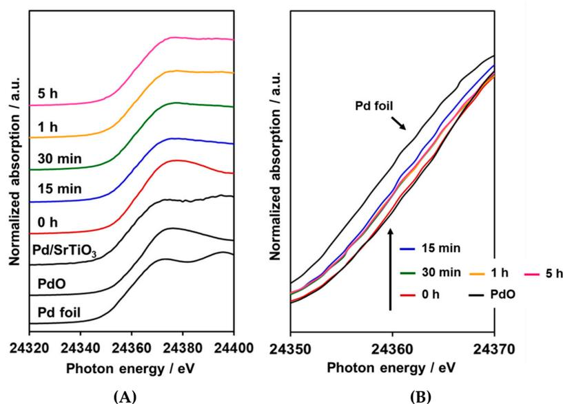
**Figure 4.** The Pd K-edge XANES spectra of PdCrO<sub>x</sub> nanoparticles (0–5 h) on SrTiO<sub>3</sub>: (A) Wide view, and (B) narrow view. The XANES spectra of Pd foil, PdO and Pd/SrTiO<sub>3</sub> as references. The order of the K-edge positions is: (Low) < Pd foil ≈ Pd/STO < 15 min < 5 h ≈ 1 h ≈ 30 min < 0 h < PdO < (high).
