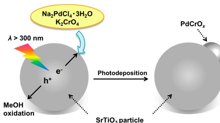
**Scheme 1.** Photochemical preparation of  $\text{PdCrO}_x$  nanoparticles on the surface of  $\text{SrTiO}_3$ .
