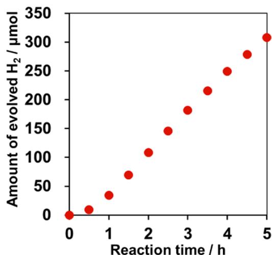
**Figure 1.** Time course of H<sub>2</sub> evolution during the photodeposition of PdCrO<sub>x</sub> nanoparticles. Reaction conditions: Catalyst, 200 mg; 10 vol% aqueous methanol solution, 100 mL; metal precursors, Pd 0.5 wt%, Cr 1.0 wt%; light source, 300 W xenon lamp ( $\lambda > 300$  nm).
