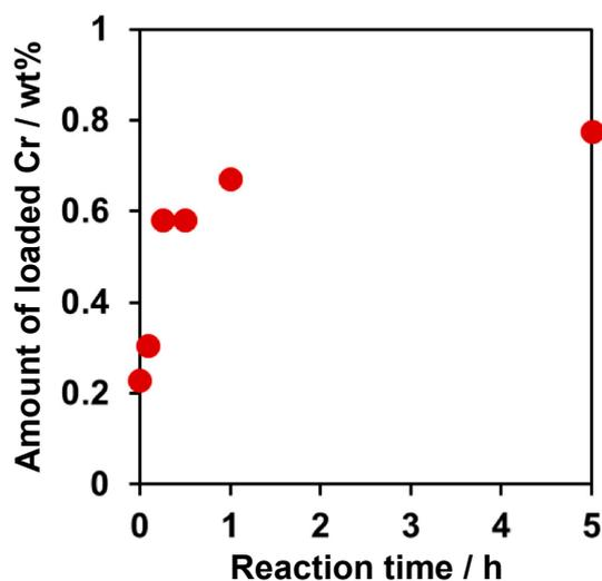
**Figure 2.** Amount of Cr contained in PdCrO<sub>x</sub>/SrTiO<sub>3</sub> at various photodeposition times.
