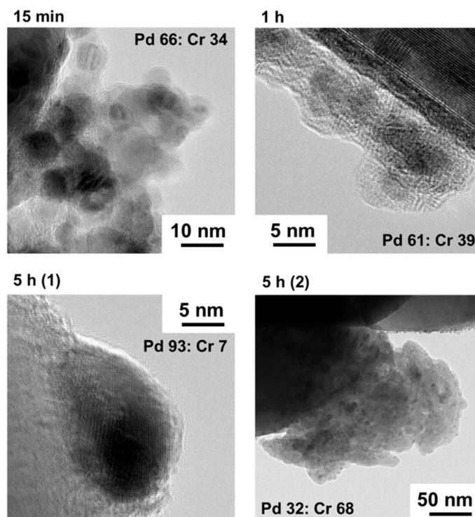
**Figure 3.** Transmission electron microscopy (TEM) images and Pd/Cr weight ratios of PdCrO<sub>x</sub>/SrTiO<sub>3</sub> prepared for various time periods (15 min, 1 and 5 h). The weight ratio was calculated from energy dispersive X-ray spectroscopy (EDX) measurements.
