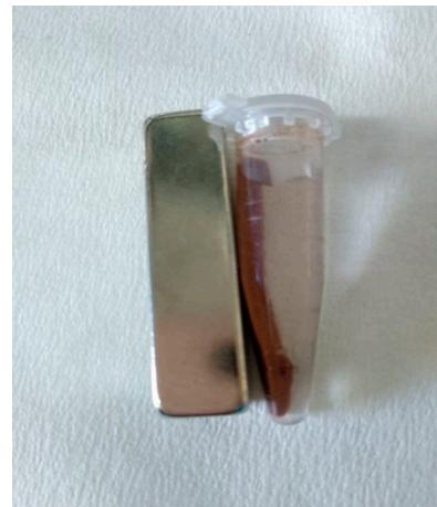
**Figure S7.** Nanobiocatalyst's magnetic separation by the use of an external magnetic field.
