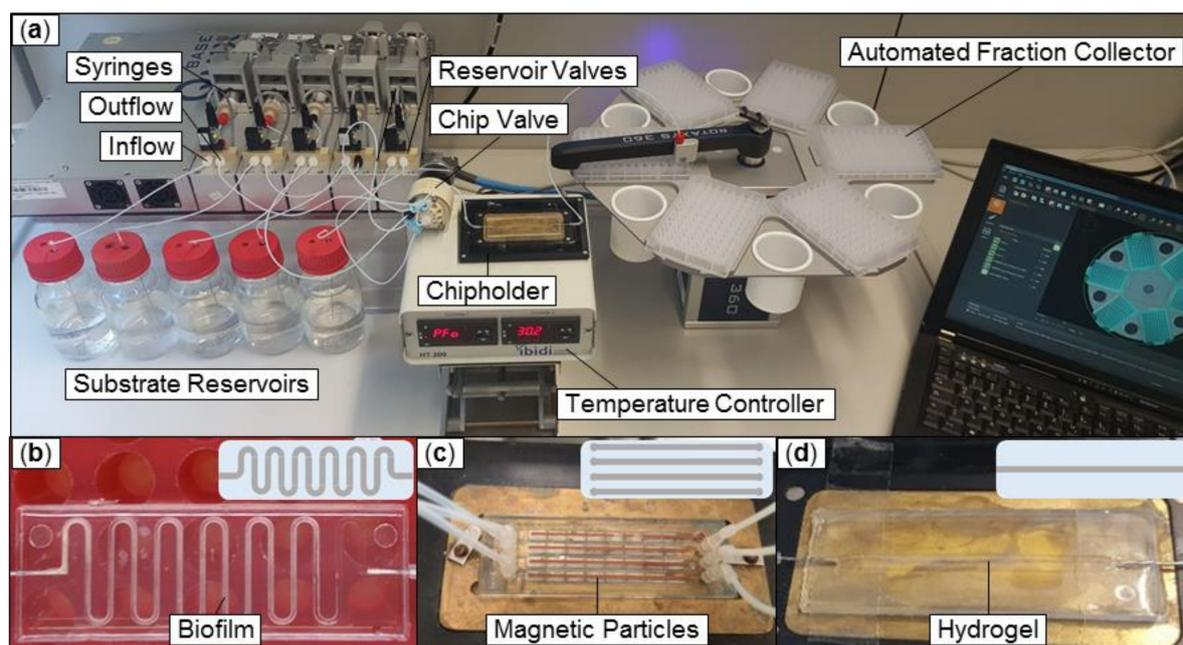
**Figure 1.** Setup for continuous flow biocatalysis using microfluidic chip reactors. (a) Overview of the microfluidic system with photo and scheme of (b) polydimethylsiloxane (PDMS) chip with meandering flow path containing a productive *Escherichia coli* biofilm. (c) polymethylmethacrylate (PMMA) chip with permanent magnets arranged beneath the flow channel holding enzyme-functionalized magnetic particles (brown). (d) PDMS chip with pure all-enzyme hydrogel in a straight flow path.
