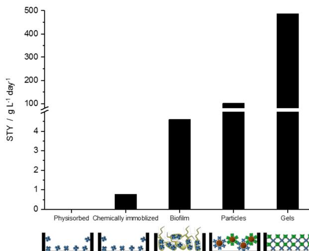
**Figure 4.** Diol **3d** space–time yields (STY) obtained for the various different flow-biocatalysis reactor modules. Schemes of the chip cross section with the immobilized biocatalyst are shown underneath the corresponding bar graphs.
