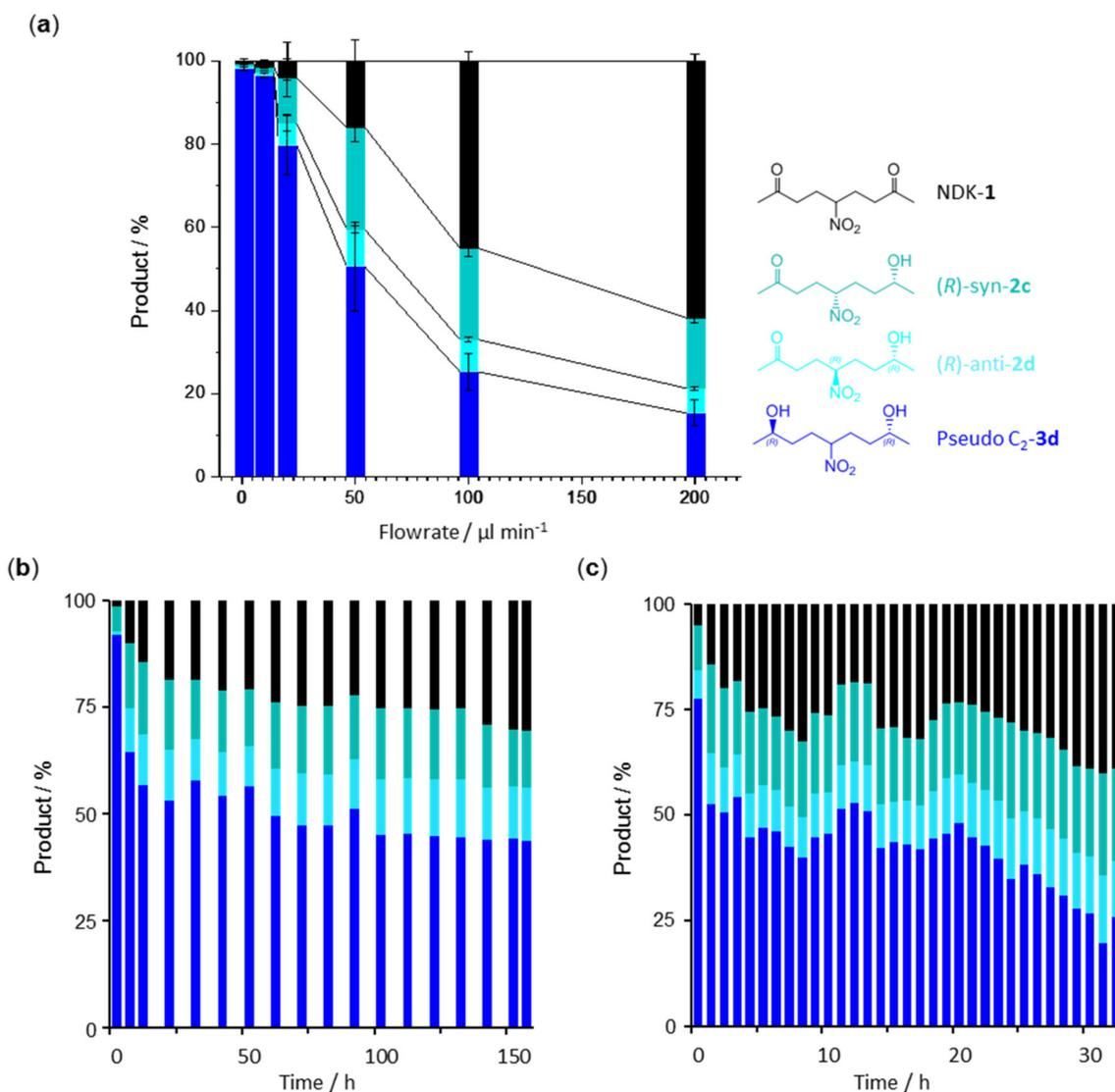
**Figure 3.** Product distributions determined in the outflow of reactor modules containing the LbADH-ST/GDH-SC hydrogel: (a) Flowrate dependency; (b) long-term time dependency with continuous NADP<sup>+</sup>-supply over >6 days (flowrate 10 µL/min); (c) time dependency with encapsulated NADP<sup>+</sup> (flowrate 10 µL/min).
