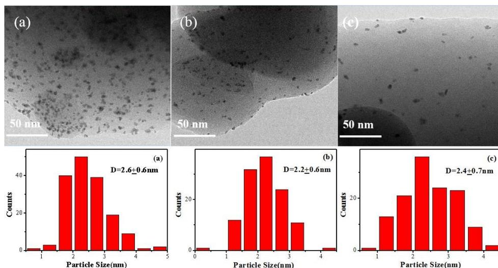
**Figure S1.** TEM images and corresponding size distribution of Pt<sub>0.8</sub>/SiO<sub>2</sub>-Shiff (a), Pt<sub>0.5</sub>/SiO<sub>2</sub>-Shiff (b) and Pt<sub>0.3</sub>/SiO<sub>2</sub>-Shiff (c).
