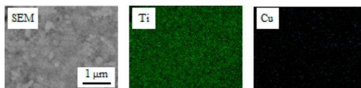
**Figure 7.** SEM-EDS element mapping images of the powder sample prepared using the  $0.500 \text{ mmol dm}^{-3}$   $\text{Cu}(\text{NO}_3)_2$  solution and heated at 573 K for 2 h.
