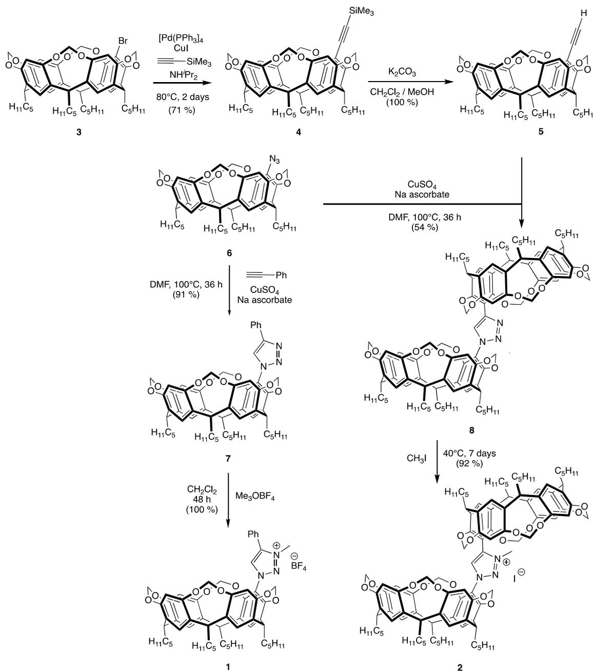
**Scheme 1.** Synthesis of the resorcinarene-based triazolium salts **1** and **2**.
