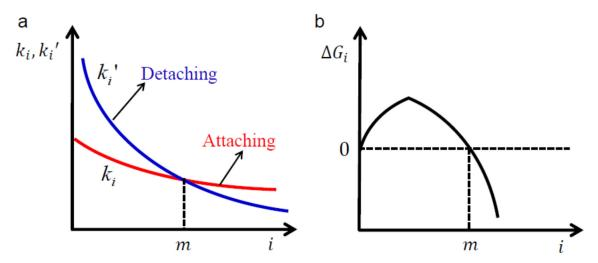
**Figure 7.** Microscopic kinetics of attaching and detaching for flexible polymer chains. (a) Variation of the rate constants of attaching and detaching with a number of monomers; (b) free energy change of formation of nuclei containing a different number of monomers. The symbol m indicates the number of monomers within the minimum stable nuclei for crystals of flexible polymers.
