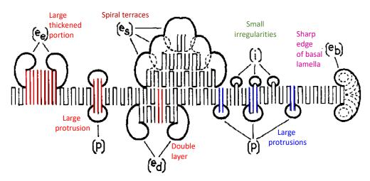
**Figure 3.** Schematic cross-section of a self-decorated poly(ethylene oxide) (PEO) crystal lamella, showing the various decorating sites, which can be encountered on PEO single crystals grown from the melt (note that the thickness of the basal lamella is about 100 times enlarged with respect to the size of the decorating units). Adapted by permission from ref. [17] Copyright 1972, Springer.
