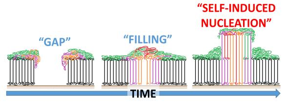
**Figure 4.** Scheme demonstrating self-induced nucleation, a new mechanism for the formation of secondary lamellar crystals, insertion of polymer chains in the impinging corner of two primary branches. Adapted from ref [22].
