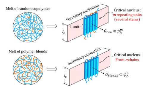
**Figure 5.** Scheme for determining the size of a critical secondary nucleus based on the crystallization kinetics of random copolymer and miscible crystallizable/amorphous polymer blends. Adapted with permission from Reference [62]. Copyright 2019, American Chemical Society.
