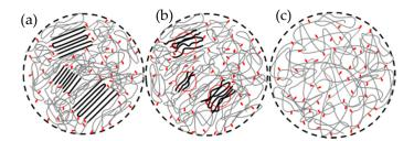
**Figure 2.** Schematics of (a) random copolymer semicrystalline structure with co-units (red dots) excluded from the crystalline regions; (b) heterogeneous, non-equilibrated melt with crystalline memory: (c) homogeneous equilibrated melt. Adapted with permission from Reference [10]. Copyright (2013) American Chemical Society.
