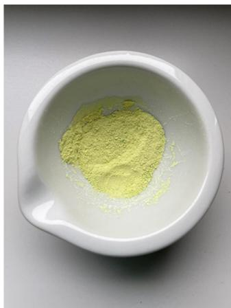
Figure 7. Appearance of the final nickel(II) perrhenate.
