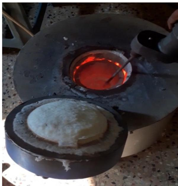
**Figure 1.** Stir casting setup.
