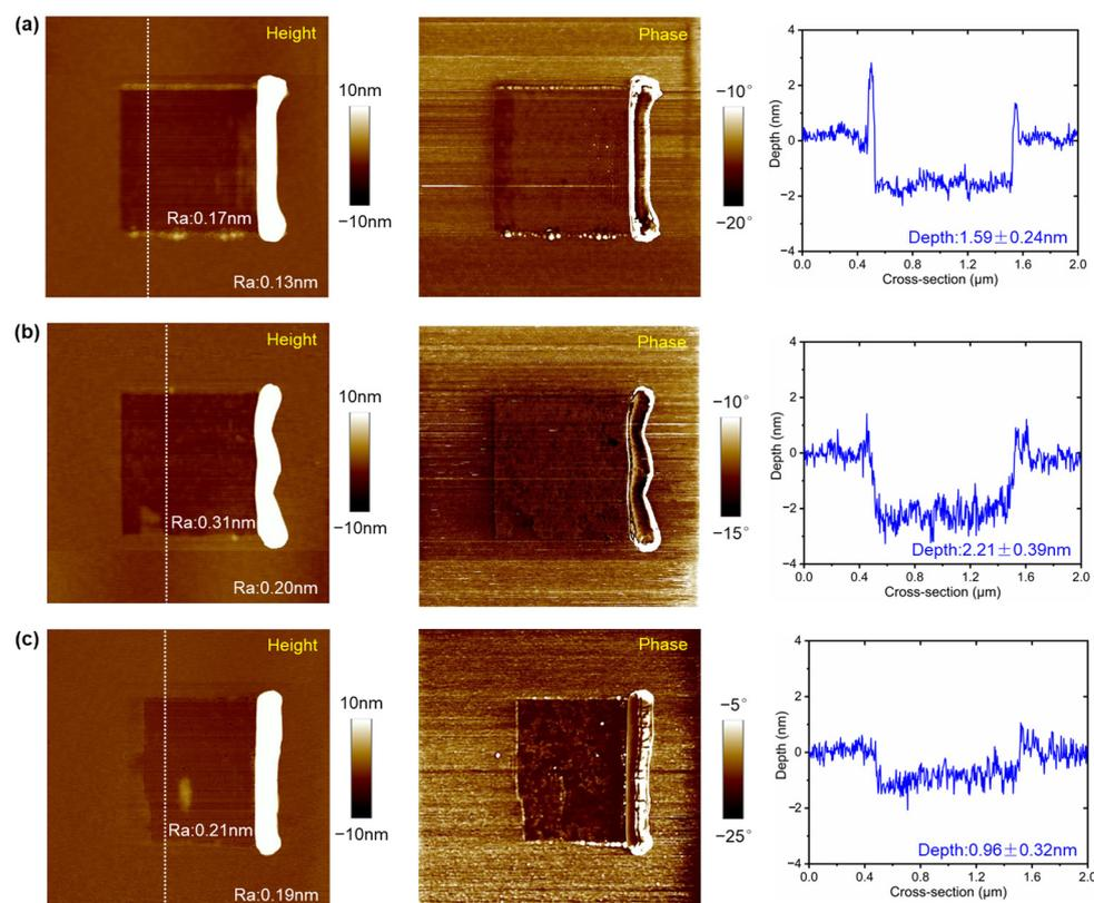
**Figure 4.** AFM images and the corresponding cross-sections of fabrication results marked in white under dynamic lithography with the driven amplitude ratio  $V_w/V_r$  of (a) 10, (b) 15 and (c) 20.
