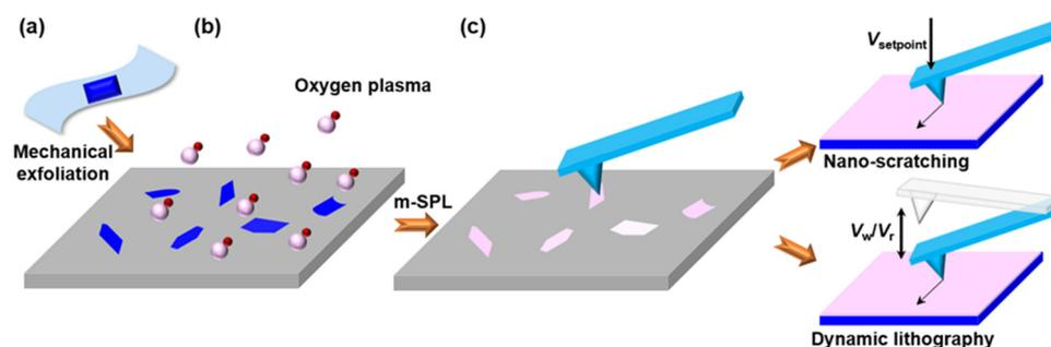
**Figure 1.** (a) Mechanical exfoliation of MoS<sub>2</sub> flakes from bulk crystal. (b) MoS<sub>2</sub> flakes treated by oxygen plasma. (c) Mechanical scanning probe lithography on MoS<sub>2</sub> flakes after oxygen plasma treatment, including nano-scratching and dynamic lithography.
