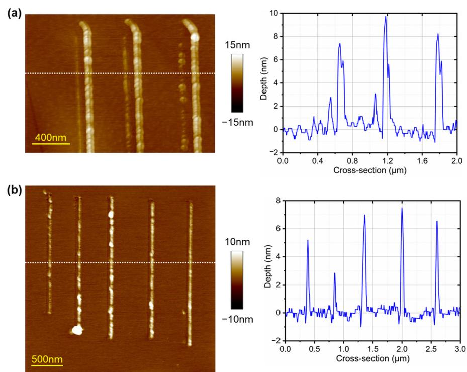
**Figure 3.** AFM images and the corresponding cross-sections of nanogrooves marked in white on a MoS<sub>2</sub> flake with oxygen plasma treatment under (a) nano-scratching and (b) dynamic lithography.
