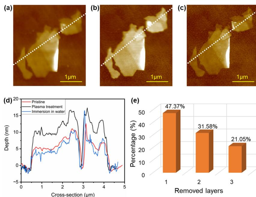
**Figure 2.** AFM images of a MoS<sub>2</sub> flake: (a) pristine flake obtained from mechanical exfoliation, (b) after oxygen plasma treatment and (c) after immersion in water for 30 s. (d) Cross-sections of the flakes in (a–c) marked in white. (e) Removal layers of MoS<sub>2</sub> flakes treated with oxygen plasma and DI water.
