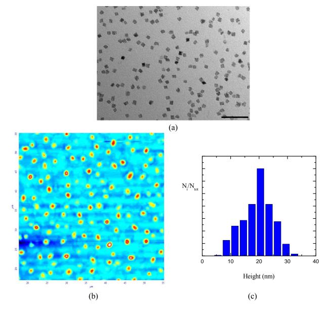
In order to check the effects of the phase on the microemulsion dynamics and/or stability and hence on the nanocrystal growth process, CdS nanocrystals were prepared in water-in-nonane microemulsions, using the same amounts of solvents and AOT as used for the heptane microemulsions.
