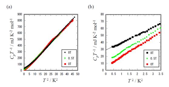
**Figure 11.** (a)Temperature dependence of heat capacity of  $\kappa$ -(MDT-TTF)<sub>2</sub>AuI<sub>2</sub> obtained under 0 T, 0.5 T, 1 T and 2 T. (b) The extended plot of  $C_pT^{-1}$  vs.  $T^2$  in the low temperature region.
