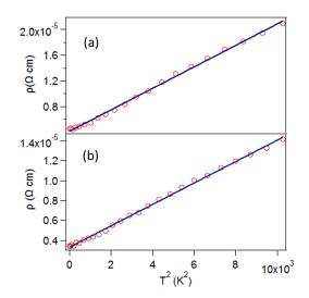
**Figure 5.**  $T^2$  power law fit of low temperature resistivity of (a) NbP and (b) TaP.
