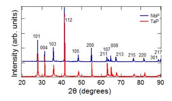
Figure 2. Room temperature X-ray diffraction pattern of NbP and TaP with reflections indicated.
