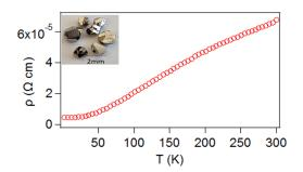
**Figure 3.** Resistivity vs. temperature of an unoriented crystal of NbP. Single crystals of NbP are shown in the inset.
