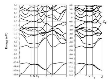
**Figure 6.** The band structure of NbP. The left panel does not include spin orbit coupling (SOC); the right panel includes SOC.
