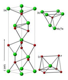
**Figure 1.** Conventional unit cell of NbP or TaP (**a**); Trigonal prismatic environment of P (**b**) and Nb/Ta (**c**).
