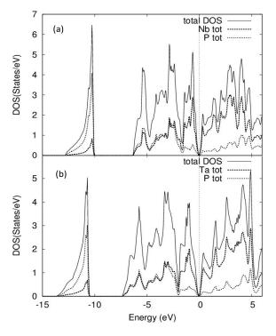
Figure 8. Non-spin polarised electronic density of states of (a) NbP and (b) TaP including SOC.
