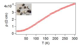
**Figure 4.** Resistivity vs. temperature of an unoriented crystal of TaP. Single crystals of TaP are shown in the inset.
