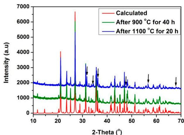
**Figure 1.** Calculated and experimental XRD of  $\text{Ba}_2\text{Zn}(\text{BO}_3)_2$ . The black arrows refer to ZnO (PDF# 79-0206).
