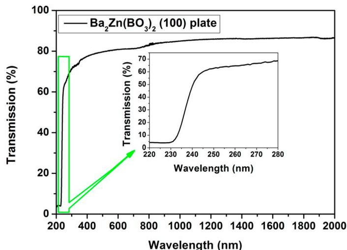
**Figure 4.** UV-vis-NIR transmission spectra of Ba<sub>2</sub>Zn(BO<sub>3</sub>)<sub>2</sub> (100) plate. Insert is enlarged UV range.
