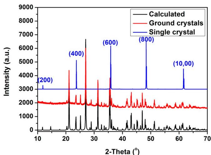
**Figure 3.** Calculated and experimental XRD patterns of  $Ba_2Zn(BO_3)_2$  crystals.
