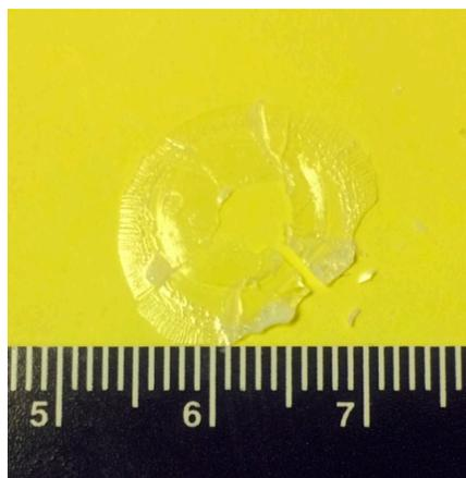
**Figure 2.** Photo of as-grown  $Ba_2Zn(BO_3)_2$  crystals. The minimum scale on the ruler is 1 mm.
