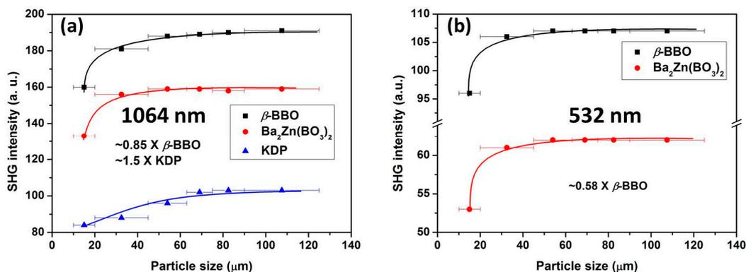
**Figure 5.** Powder SHG measurement of polycrystalline Ba<sub>2</sub>Zn(BO<sub>3</sub>)<sub>2</sub> at the fundamental wavelengths of (a) 1064 nm (b) 532 nm. Note the curves are drawn to guide the eye and are not a fit to the data.
