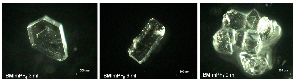
Figure 6. Video microscope images of sucrose crystals precipitated from the MeOH extraction solution of A. gigas (solvent volume of 3 mL) at varied concentrations of BMImPF 6 anti-solvent changes using crystallization techniques.
