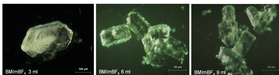
Figure 5. Video-microscope images of sucrose crystals obtained from the MeOH extraction solution of A. gigas (solvent volume of 3 mL) under BMImBF 4 anti-solvent concentration change using crystallization techniques.
