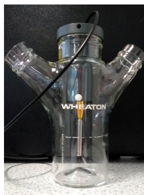
Figure 2. Photograph of the hydrophone arrangement within the Celstir vessel set-up for ultrasonic intensity measurement.
