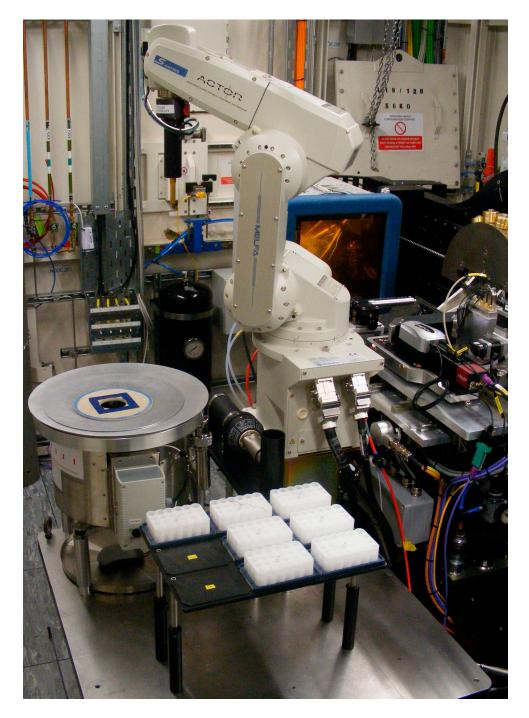
**Figure 8.** The robotic sample changer. The Dewar for storing unipucks is shown to the left of the robotic arm while the trays for holding sample mounts under ambient conditions are shown in the foreground. The aperture in the sliding lid of the Dewar is indicated by a blue square inside a blue circle for the image-recognition system. The camera for locating the lid aperture is mounted above the robot table and not shown here.
