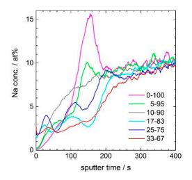
**Figure 6.** Comparison of the Na-concentration depth profiles in porous silica coatings with 5, 10, 17, 25, and 33 mol % CeO<sub>2</sub>. Curing conditions were 60 min at 350 °C.
