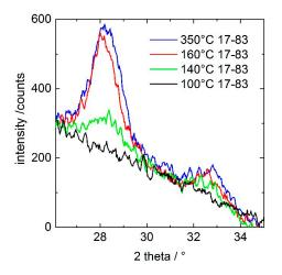
**Figure 3.** Evolution of the (111) and (200) diffraction peaks of cubic ceria (at approximately  $28^{\circ}$  and  $33^{\circ}$  2 $\theta$ ) during in situ GIXRD in a high-temperature chamber heated at 10 K/min from room temperature up to  $350 \,^{\circ}$ C.
