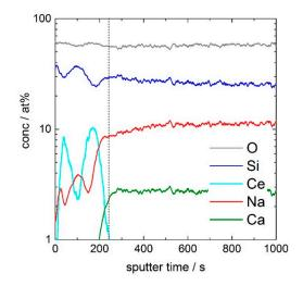
**Figure 4.** Secondary neutral mass spectrometry (SNMS) depth profile of the elements: oxygen (O), silicon (Si), cerium (Ce), sodium (Na), and calcium (Ca) of the 17–83 coating on low-iron soda-lime glass. Vertical dashed line at 240 s indicates the interface of the coating and the substrate glass. Curing conditions were 60 min at 350  $^{\circ}$ C.
