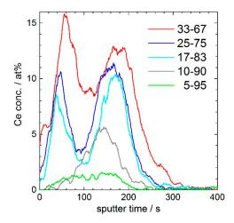
**Figure 5.** Comparison of the Ce-concentration depth profiles in porous silica coatings with 5, 10, 17, 25, and 33 mol % CeO<sub>2</sub>. Curing conditions were 60 min at 350 °C.
