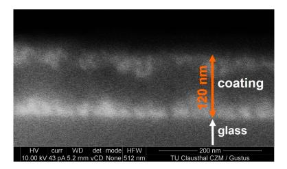
**Figure 7.** Fracture surface of the 17–83 coating on low-iron soda-lime glass by backscattered electron imaging (FESEM). The location of the heavier ceria crystals is indicated by the brighter regions in the image.
