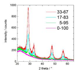
**Figure 2.** Grazing incidence X-ray diffraction (GIXRD) patterns of porous silica coatings with 5, 17, and 33 mol % CeO<sub>2</sub> on low-iron soda-lime glass. Curing conditions were 60 min at 350 °C.
