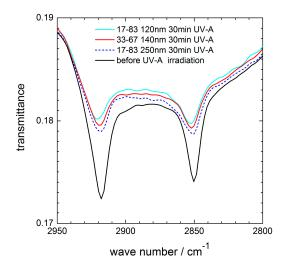
**Figure 9.** IR-absorption bands of the symmetric stretching modes of the CH<sub>2</sub> group at 2923 and 2853 cm<sup>-1</sup> of a stearic acid film on CeO<sub>2</sub>-containing porous silica coatings of 120, 140, and 250 nm thickness on low-iron soda-lime glass before and after 30 min of UV-A irradiation. CeO<sub>2</sub> concentration was 17 mol % for the 120 and 250 nm coating and 33 mol % for the 140 nm coating.
