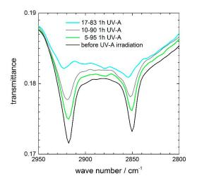
**Figure 8.** IR-absorption bands of the symmetric stretching modes of the CH<sub>2</sub> group at 2923 and 2853 cm<sup>-1</sup> of a stearic acid film on 120 nm porous silica coatings containing 5, 10, and 17 mol % CeO<sub>2</sub> on low-iron soda-lime glass before and after 1 h of UV-A irradiation.
