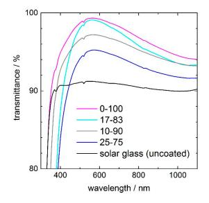
**Figure 1.** UV–Vis–NIR transmittance spectra of antireflective (AR) coatings from porous silica, containing 10, 17, and 25 mol % CeO<sub>2</sub>, on low-iron soda-lime glass in comparison to uncoated glass. Curing conditions were 60 min at 350 °C.
