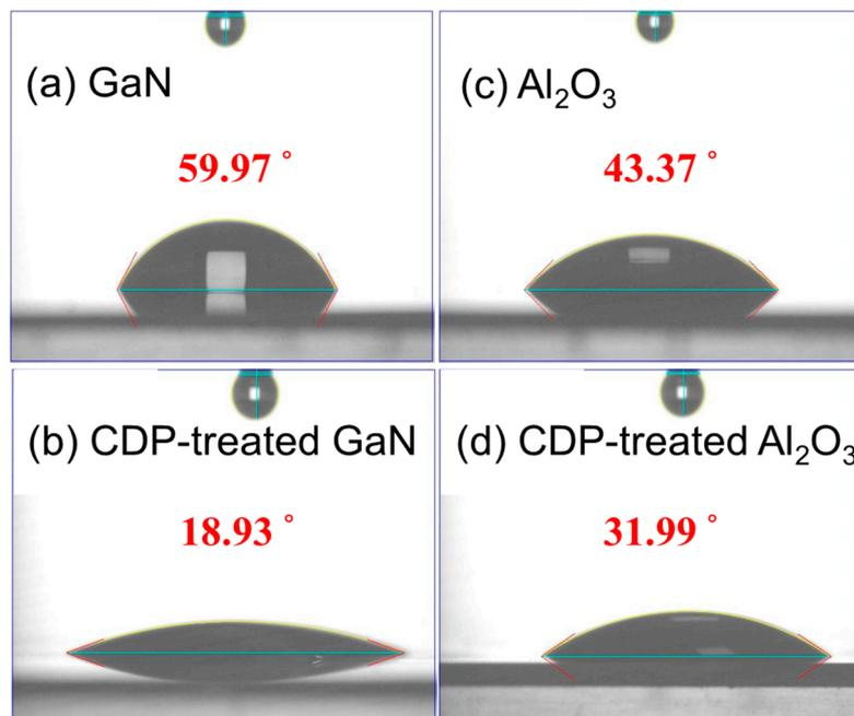
**Figure 2.** Contact angle of DI water performed on (a) GaN; (b) corona-discharge plasma (CDP)-treated GaN; (c) Al<sub>2</sub>O<sub>3</sub>; and (d) CDP-treated Al<sub>2</sub>O<sub>3</sub>.
