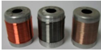
**Figure 2.** Spools with glass-coated microwires produced from different metallic alloys.
