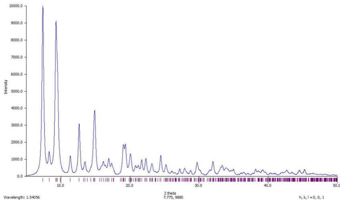
**Figure SI 9.** Simulation of the PXRD of **1** monocystal structure with FWHM 0.3.
