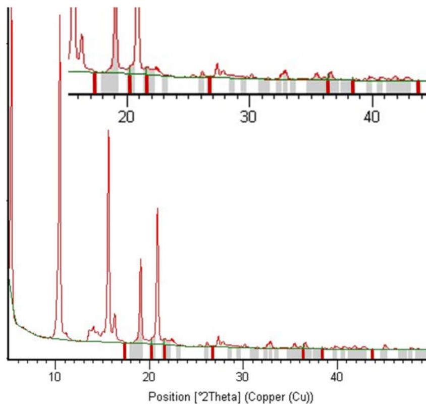
**Figure SI 5.** Powder X-ray diffraction (PXRD) of **1** compared with Mn(II) in MnO pattern. Inset: a zoom of the spectrum is placed for clarity.
