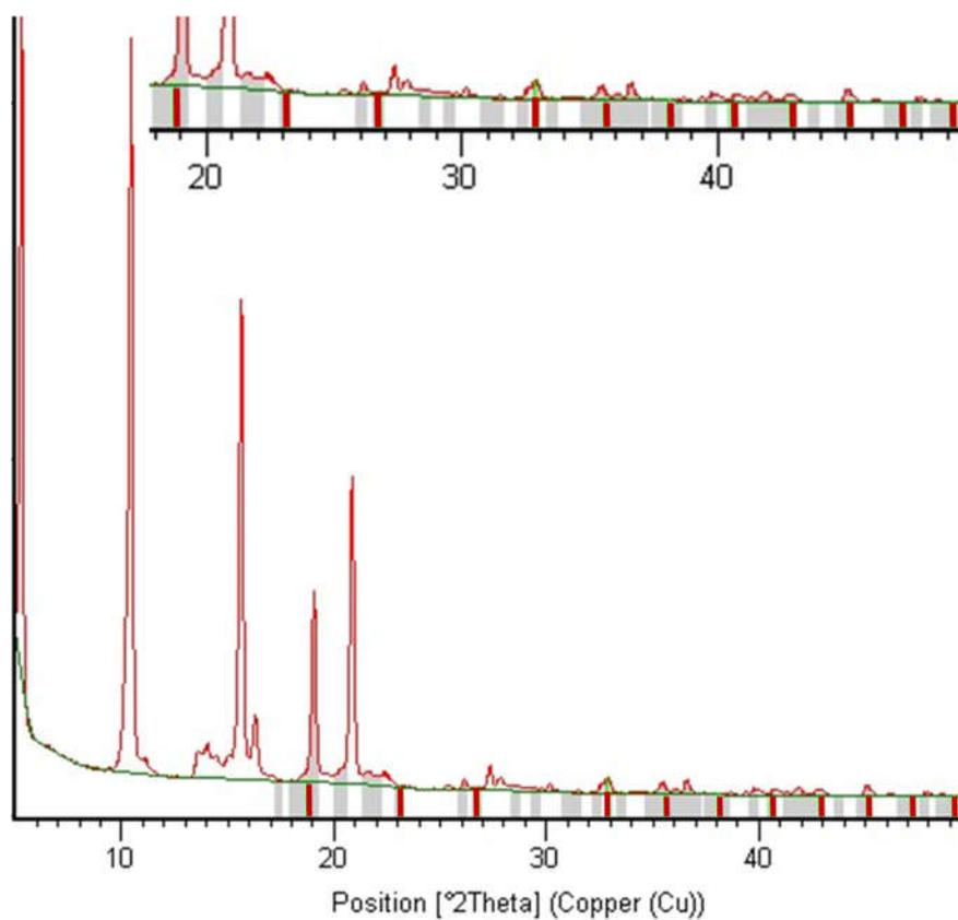
**Figure SI 6.** PXRD of **1** compared with Mn(III) in Mn<sub>2</sub>O<sub>3</sub> pattern. Inset: a zoom of the spectrum is placed for clarity.
