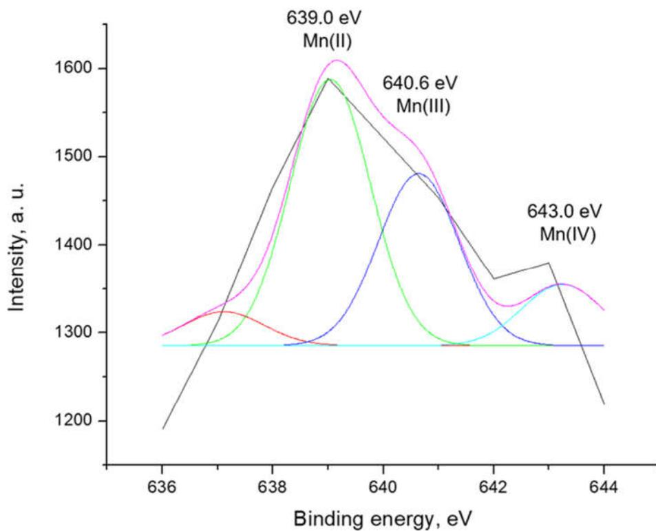
**Figure SI-3.** Mn2p<sub>3/2</sub> spectra of Mn complex. A model of three gaussian curves fit to reproduce the experimental results.
