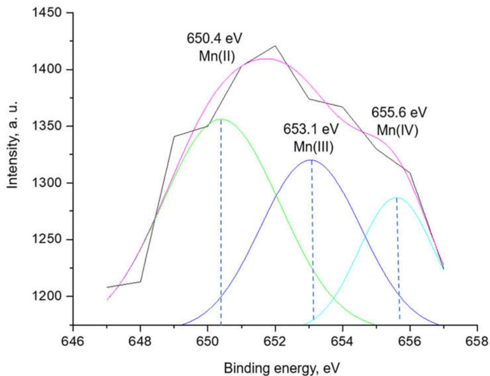
**Figure SI4.** Mn2p  $1/2$  spectra of Mn complex. A model of three Gaussian curves fit to reproduce the experimental results.
