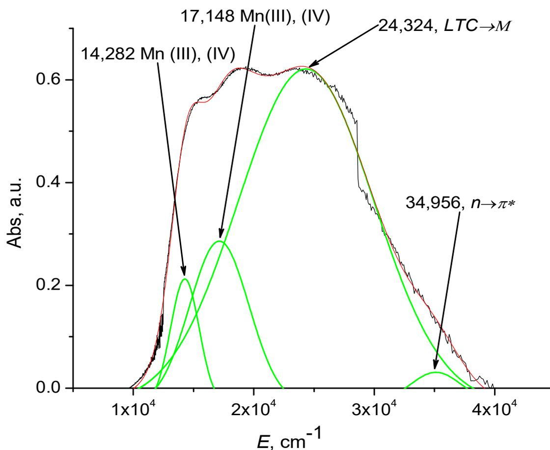
**Figure SI-1.** UV-Vis spectrum of 1 on polycrystalline sample showing the electronic transitions at typical reported energies for Mn(III) and Mn(IV). .
