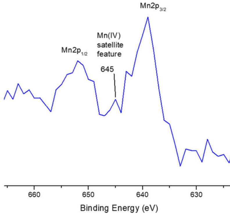
**Figure SI-2.** Mn2p spectra of Mn complex. MnO has a satellite feature (~647 eV), which is not present for either Mn<sub>2</sub>O<sub>3</sub> or MnO<sub>2</sub>.
