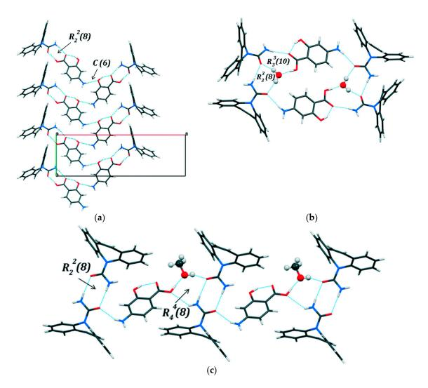
**Figure 18.** Hydrogen bond interaction present in (**a**) 1:1 CBZ-PAS cocrystal; (**b**) 2:1:1 CBZ-PAS-water and (**c**) 2:1:1 CBZ-PAS-methanol structure. Adapted with permission from *CrystEngComm*, 2017, 19, 4273–4286. Copyright 2017, The Royal Society of Chemistry.
