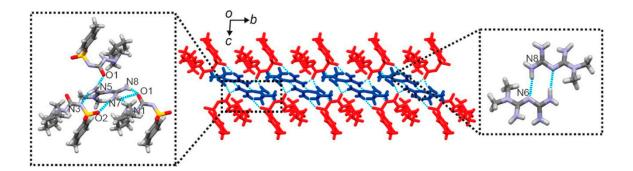
**Figure 29.** Infinite 1D hydrogen bond chain of MET-GLI crystal along the *a*-axis (blue for MET and red for GLI). Detailed interaction between MET-MET (**right**) and MET-GLI (**left**) presented in default color according to the different elements. Blue-dashed lines indicate hydrogen bonds. Adapted with permission from *Crystal Growth & Design*, 2016, 16, 3577–3581. Copyright 2016, American Chemical Society.
