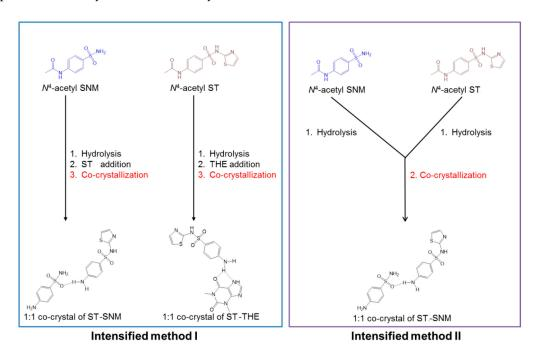
**Figure 36.** Intensified method for cocrystal preparation. Adapted with permission from *Cryst. Growth Des.*, DOI: 10.1021/acs.cgd.7b01197. Copyright 2018, American Chemical Society.
