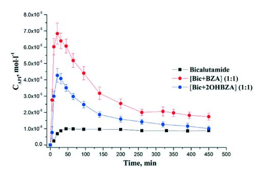
**Figure 10.** Dissolution profiles for the cocrystals (Bic + BZA and Bic + 2OHBZA) and pure bicalutamide in the pH 7.4 phosphate buffer at 25 °C. Adapted with permission from *CrystEngComm*, 2016, **18**, 4818–4829. Copyright 2016, The Royal Society of Chemistry.
