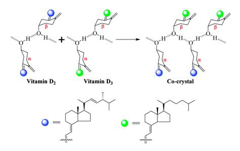
**Figure 42.** Design and synthesis of  $VD_2$ - $VD_3$  cocrystal. Blue and green ball represent the substituent groups present in  $VD_2$  and  $VD_3$ . Adapted with permission from *Chemical Communications*, 2016, 52, 3572–3575. Copyright 2016, The Royal Society of Chemistry.
