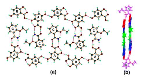
**Figure 20.** (a) A zipper like structure in EA:GA cocrystal Form I. (b) 3D crystal packing showing the EA molecule connecting the zipper-like network. Adapted with permission from *CrystEngComm*, 2009, 11, 1823–1827. Copyright 2009, The Royal Society of Chemistry.
