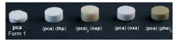
**Figure 38.** Tablet resulting from compression experiments involving paracetamol (pca form I) and cocrystals with theophylline (thp), naphthalene (nap), oxalic acid (oxa), and phenazine (phe) respectively. Adapted with permission from *Adv. Mater.* 2009, 21, 3905–3909. Copyright 2009, John Wiley & Sons.
