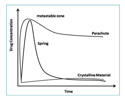
**Figure 2.** The 'spring and parachute' approach to promoting and maintaining supersaturation of poorly soluble drugs. Adapted with permission from *Cryst. Growth Des.*, 2011, 11 (7), 2662–2679. Copyright 2011 American Chemical Society.
