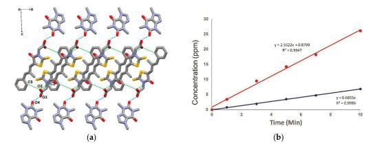
**Figure 16.** (a) Layered structure of 1:1 caffeine-epalrestat cocrystal connected through O–H…O hydrogen bond. Hydrogen atoms were removed for clarity. (b) Intrinsic dissolution rate of caffeine-epalrestat cocrystal (red) compared with pure epalrestat drug (blue). Adapted with permission from *CrystEngComm*, 2017, 19, 2614–2622. Copyright 2017, The Royal Society of Chemistry.
