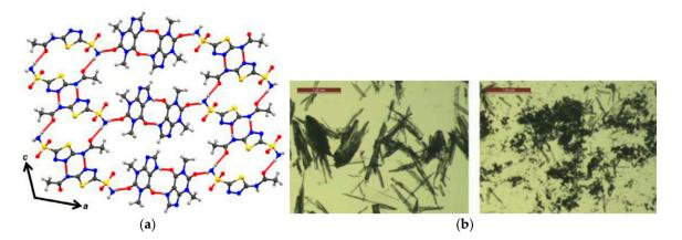
**Figure 41.** (a) Hydrogen bond interaction present in theophylline–acetazolamide cocrystal structure. (b) Plastic deformation in theophylline-acetazolamide cocrystal before (**left**) and after (**right**) application of mechanical stress. Adapted with permission from *CrystEngComm*, DOI: 10.1039/C7CE01915G. Copyright 2018, The Royal Society of Chemistry.
