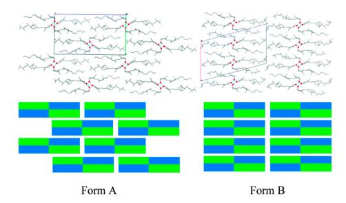
**Figure 43.** Packing arrangement of cocrystal form A and form B viewed along the helix structure. Adapted with permission from *Chemical Communications*, 2016, 52, 3572–3575. Copyright 2016, The Royal Society of Chemistry.
