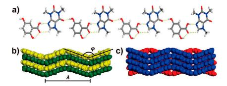
**Figure 12.** (a) Acid-imidazole dimer and hydroxyl–amide dimer between 25DHBA and caffeine resulting a 1D polymeric chain. (b,c) Stacked packing of the 1D polymer sustained by weak C–H…O hydrogen bond. Adapted with permission from *Cryst. Growth Des.*, 2009, 9 (4), 1932–1943. Copyright 2009, American Chemical Society.
