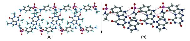
**Figure 14.** N–H···O and N–H···N hydrogen bond connecting sulfacetamide and coformer (**a**) caffeine and (**b**) theophylline in the respective cocrystals. Adapted with permission from *CrystEngComm*, 2014, *16*, 5859–5869. Copyright 2014, The Royal Society of Chemistry.
