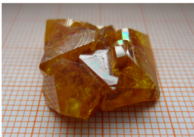
Figure 1. As-grown PLN-0.07PT crystal using the top-seeded solid solution growth (TSSG) method.
