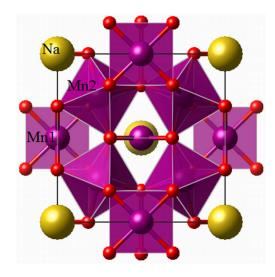
**Figure 1.** [100] projection of the quadruple perovskite structure having general formula  $AA'_{3}B_{4}O_{12}$ . In the present case, A, A' and B correspond to the Na1, Mn1 and Mn2 sites, respectively.
