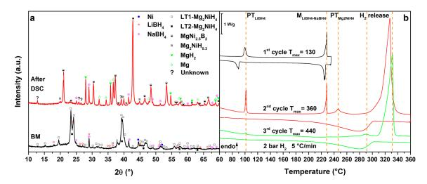
**Figure 4.** (a) PXD of the ball milled MgNiLiNa (black, down) and after cycling in HP-DSC (red, up); (b) HP-DSC cycling of MgNiLiNa at 5 °C/min under a static pressure of 2.2 bar of H<sub>2</sub>.
