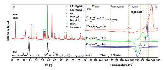
**Figure 5.** (a) PXD of the ball milled MgNiLiMg (black, down) and after cycling in HP-DSC (red, up); (b) HP-DSC cycling of MgNiLiMg at  $5 \, ^{\circ}$ C/min under a static pressure of 2.2 bar of H<sub>2</sub>.
