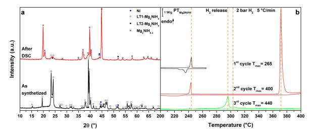
**Figure 1.** (a) PXD of the as synthetized  $Mg_2NiH_4$  (black, down) and after cycling in HP-DSC (red, up); (b) HP-DSC cycling of  $Mg_2NiH_4$  at 5 °C/min under a static pressure of 2.2 bar of  $H_2$ .
