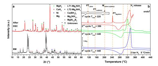
**Figure 6.** (a) PXD of the ball milled MgNiLiCa (black, down) and after cycling in HP-DSC (red, up); (b) HP-DSC cycling of MgNiLiCa at 5 °C/min under a static pressure of 2.2 bar of H<sub>2</sub>.
