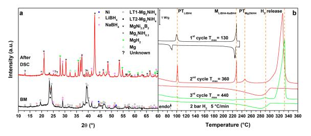
**Figure 3.** (a) PXD of the ball milled MgNiLiNa (black, down) and after cycling in HP-DSC (red, up); (b) HP-DSC cycling of MgNiLiNa at  $5 \, ^{\circ}$ C/min under a static pressure of 2.2 bar of H<sub>2</sub>.
