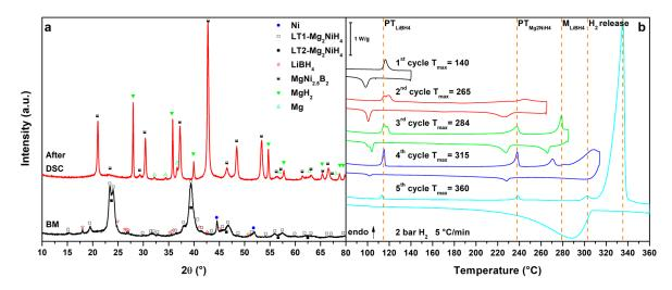
**Figure 2.** (a) PXD of the ball milled MgNiLi system (black, down) and after cycling in HP-DSC (red, up); (b) HP-DSC cycling of MgNiLi at 5 °C/min under a static pressure of 2.2 bar of H<sub>2</sub>.
